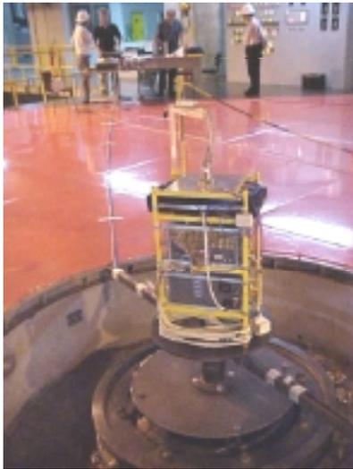
Figure 10 – Measurement Control unit at the generator top
