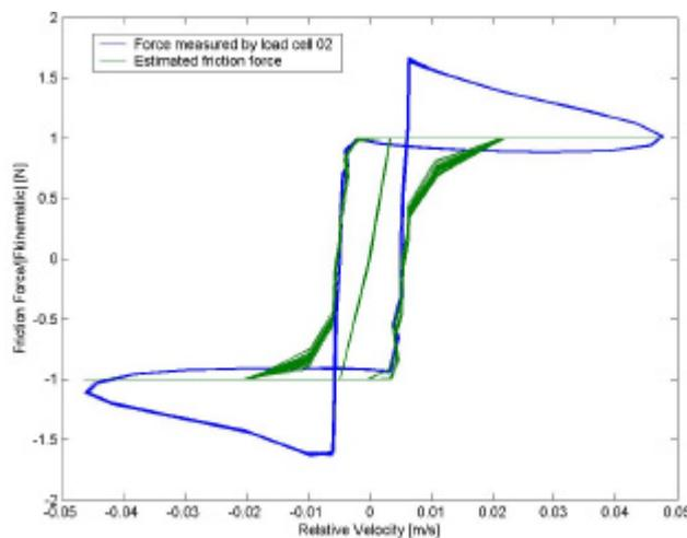
Figure 12. Behavior of nonlinear friction model and force measured by load cell 02 from group test A, with 18 Hz harmonic excitation force
