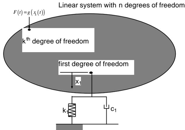
Figure 4. Linear system subjected to a nonlinear force.
