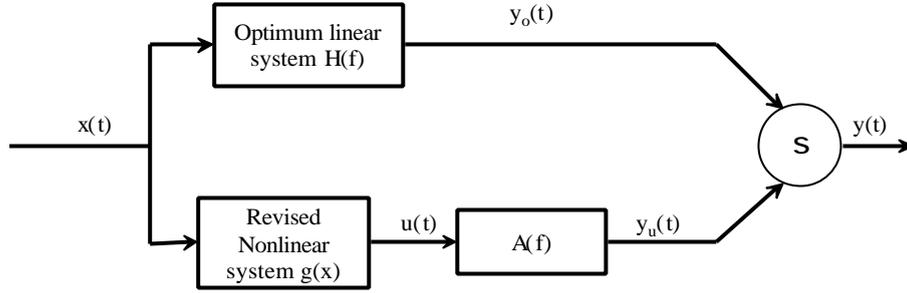
Figure 2. Nonlinear MISO system with uncorrelated inputs.
