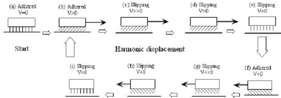
Figure 6. Schematic diagram of the friction model.
