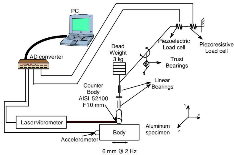
Figure 13. Experimental apparatus and the instrumentation chain used in reciprocating wear tests.
