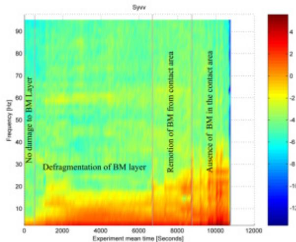
Figure 19. Frequency band from 0 to 100 Hz to experiment group B class III.
