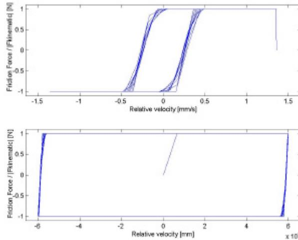
Figure 7. Behavior of nonlinear friction model.
