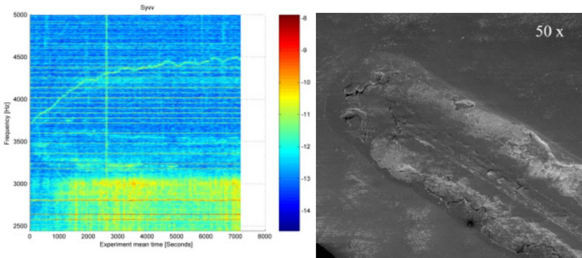
Figure 16. Nonlinear MISO results and SEM images from Class II experiments. (BM medium wear)
