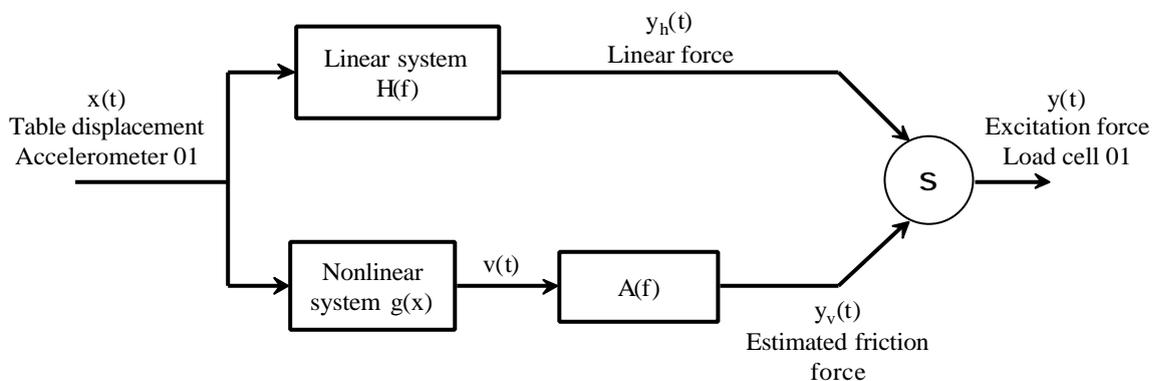
Figure 9. Nonlinear system configuration to group tests A.
