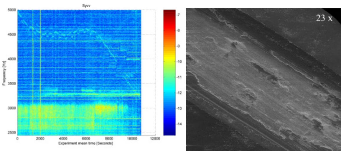
Figure 17. Nonlinear MISO results and SEM images from Class III experiments. (aluminum wear)
