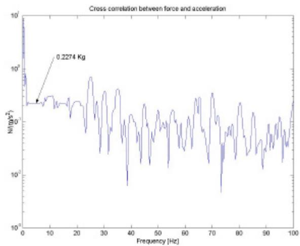
Figure 10. Cross correlation between the signals of accelerometer 01 and load cell 02.
