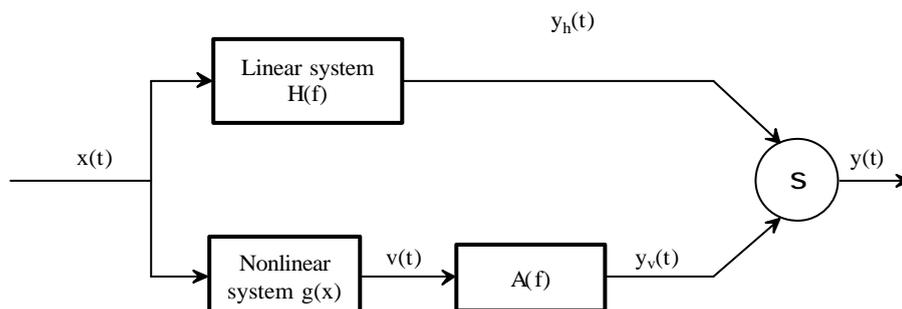
Figure 1. Nonlinear MISO systems block diagram.
