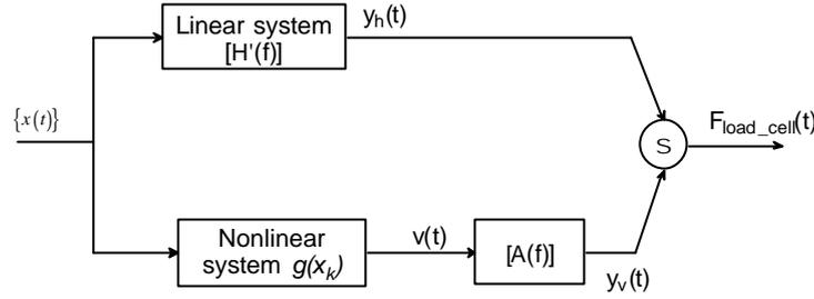
Figure 5. MISO system used to indirectly determine the nonlinear force.
