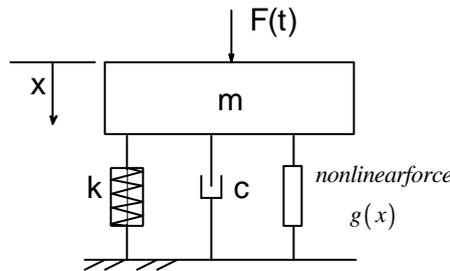
Figure 3. One degree of freedom mechanical system with a nonlinear device.
