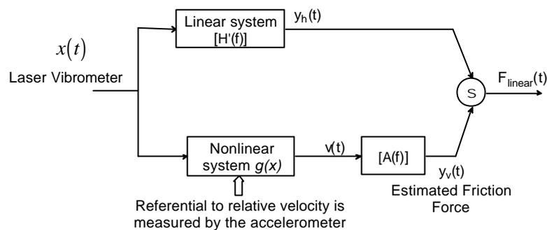
Figure 14. Nonlinear MISO system used to the reciprocating wear tests.
