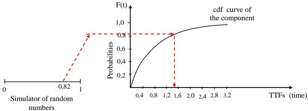
Figure 1. Determining of TTFs (time to fail) of each component - graphic representation
