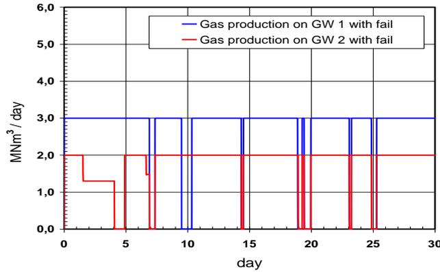
Figure 6. Gas production on the wells GW1 and GW2 taking into account random failures.
