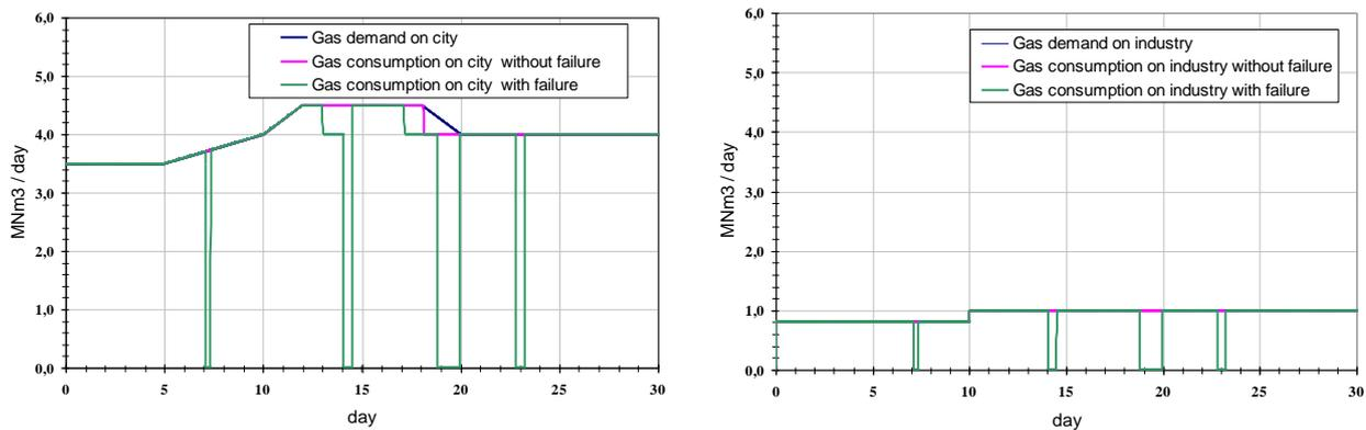
Figure 7. Left graph: gas demand along with gas consumption on City (without and with failures). Right graph: gas demand along with gas consumption on Industry (without and with failures).
