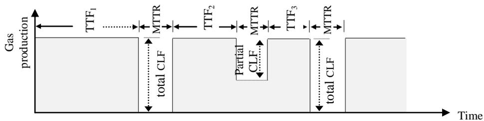
Figure 2. Impact of failures events upon the gas flow passing through a component.
