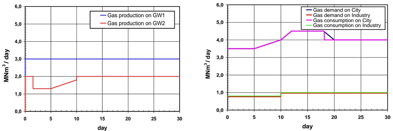
Figure 5. Gas production on the wells GW1 and GW2 (left) and gas demand along with gas consumption on the City and the Industry (right), without taking into account random failures.
