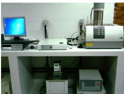
**Figura 2 - Netzsch MicroFlash LFA 457 operando no LAMET**
