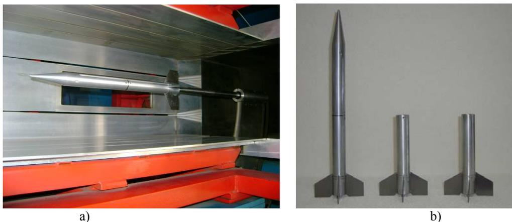
Figure 3. a) Second stage model at the test section. b) From left to right, models with fins at  $0^\circ$ ,  $2.5^\circ$  and  $5^\circ$ .
