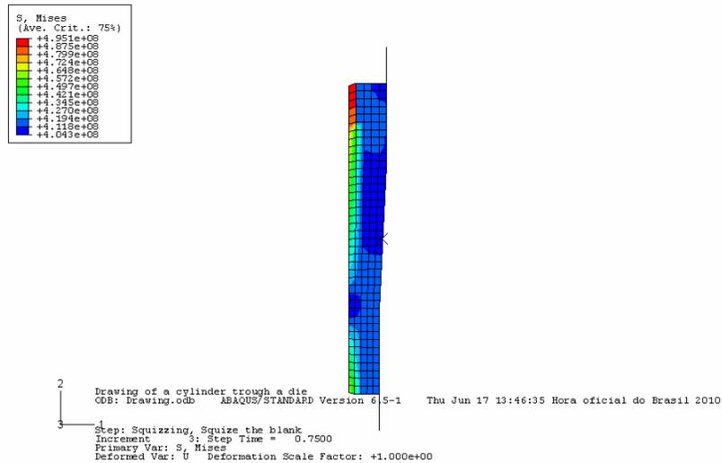
Figure 2. Intermediate deformed shape of material during process
