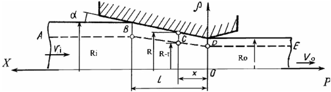
Figure 1 Geometrical and kinematics parameters of the drawing process
