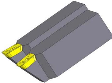
Figure 1. Drawing of toolholders used in the trials.
