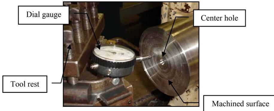
**Figure 5. Measurement of the machined surface profile using a dial gauge.**
