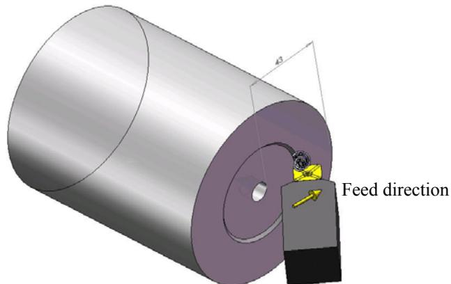
**Figure 4. Cutting geometry configuration during face turning.**
