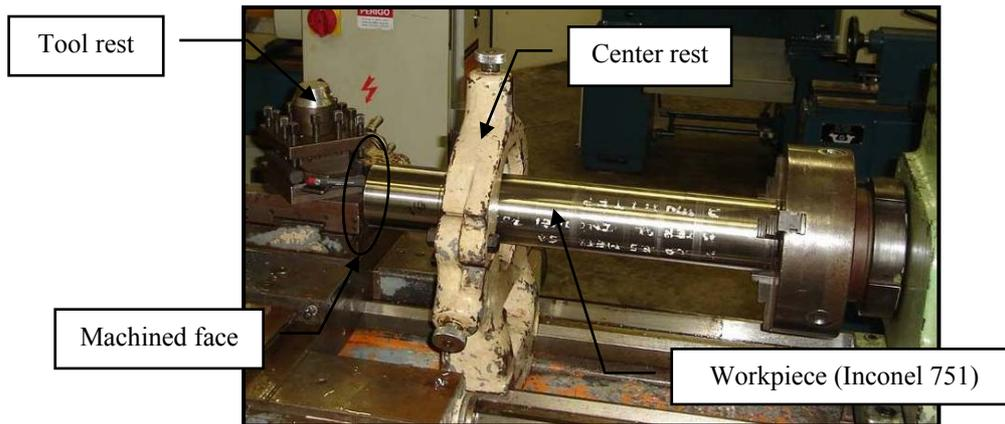
**Figure 3. Workpiece set on the conventional lathe.**
