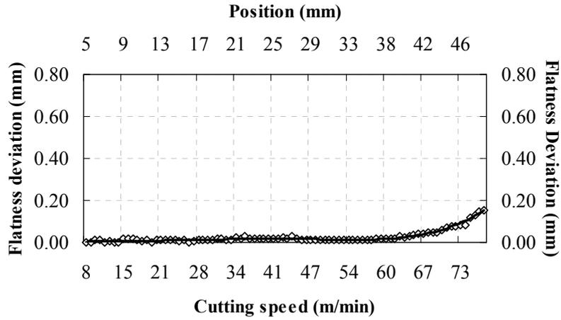
Figure 7 – Machined surface profile after machining at condition 1.
