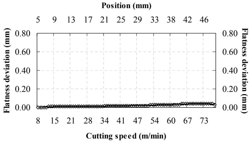
Figure 11 – Machined surface profile after machining at condition 5.
