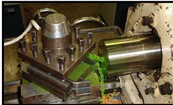
**Figure 6. Application of the cutting fluid during wet trials.**
