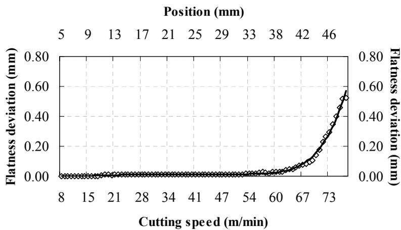
Figure 9 – Machined surface profile after machining at condition 3.
