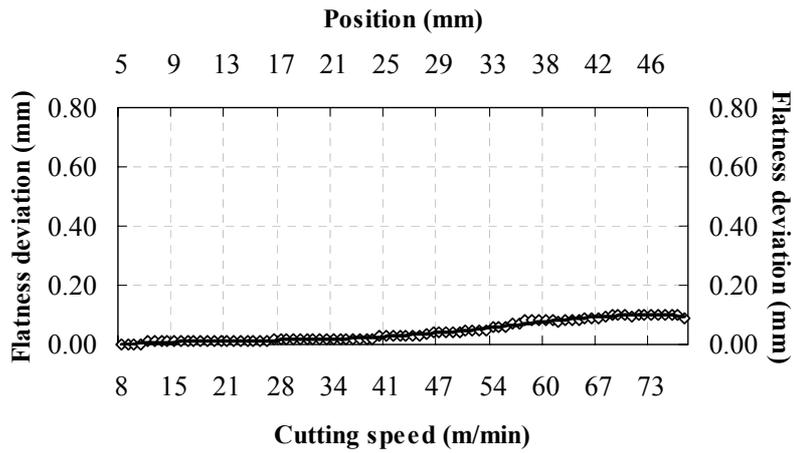
Figure 12 – Machined surface profile after machining at condition 6.
