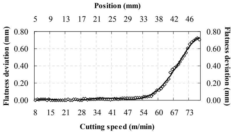
Figure 8 – Machined surface profile after machining at condition 2.
