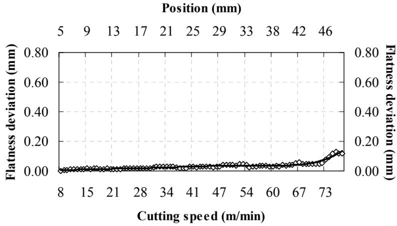
Figure 10 – Machined surface profile after machining at condition 4.
