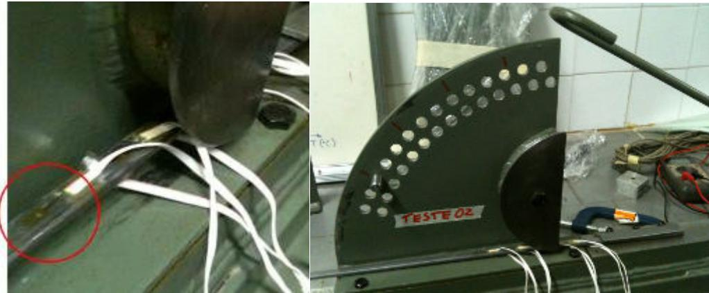
Figure 2 – Strain gages bonded on tensile armor specimen.
