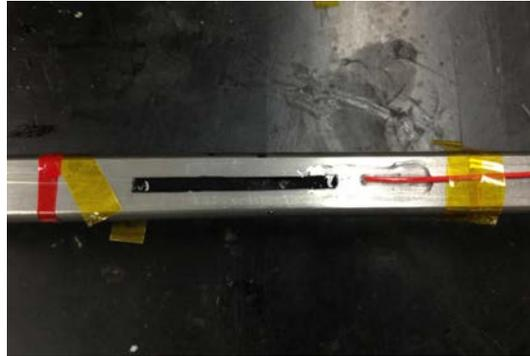
Figure 11– FBG sensor instrumentation.
