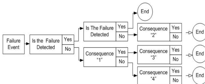
Figure 2. Cause-Consequence Diagram Logical Notation
