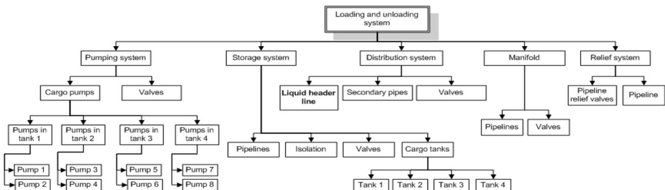
Figure 4. Functional tree for the loading and unloading system
