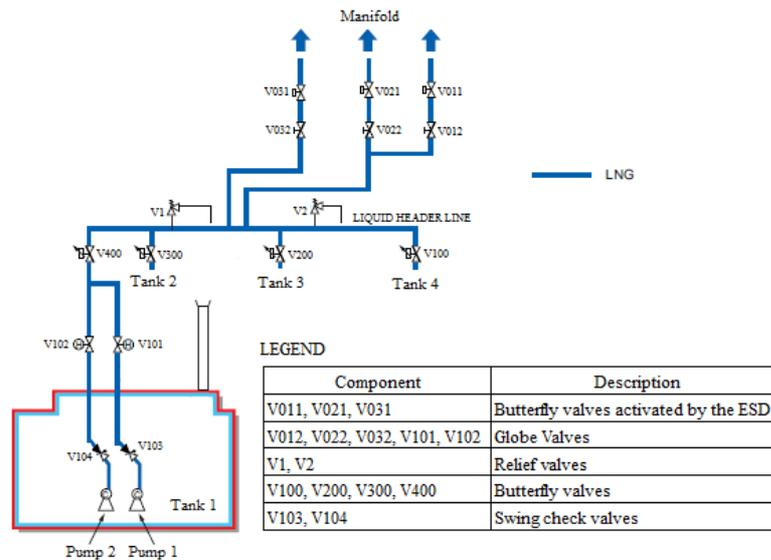
Figure 5. Cargo system diagram
