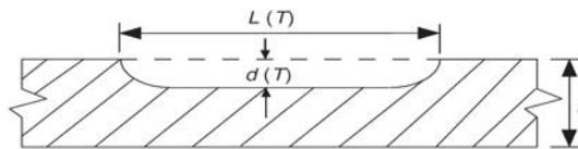
Figure 3. Pipeline wall section with an idealized corrosion defect (Qian *et al*, 2011).
