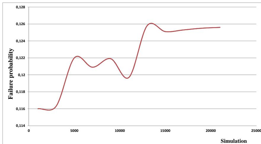
Figure 8. Probability of failure ( $P_f$ ) as a function of Monte Carlo simulation cycle for 30 operating years
