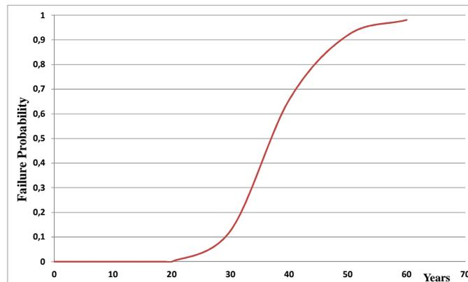
Figure 6. Probability of failure ( $P_F$ ) versus Exposure periods ( $T$ ) for 6.35mm pipe thickness
