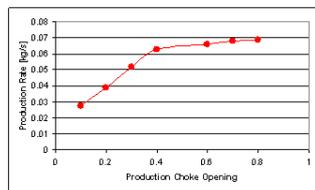
Figure 11. Production rate with respect to static choke opening.
