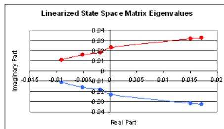
Figure 9. Eigenvalues of the linear system for different choke settings.
