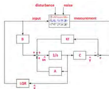
Figure 12. LQG controller and plant (Skogestad and Postlethwaite, 2005) - modified.
