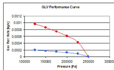
Figure 14. Approximated conventional gas lift valve performance curve.
