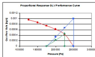
Figure 15. Simplified Proportional Response gas lift valve performance curve.
