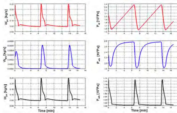
Figure 3. Production rates and pressures of a well under casing-heading.
