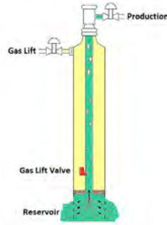
Figure 1. Gas Lift Oil Well (Eikrem *et al.*, 2008) - modified.
