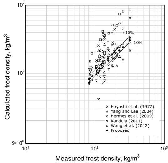
Figure 4. Comparison between experimental and calculated frost density
