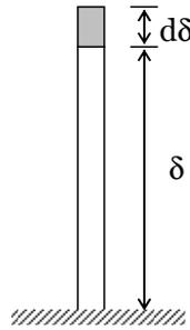
Figure 1. Schematic representation of the growth of a frost column
