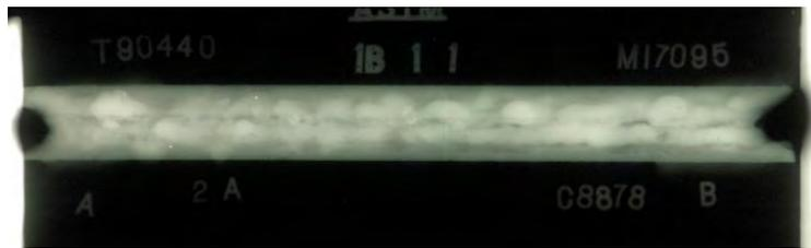
Figure 10. X-ray result for butt weld for S275 steel
