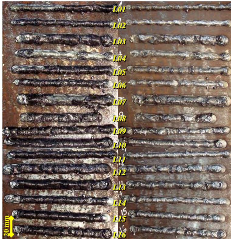
Figure 5. Bead appearance just after welding (left) and after manual brushing (right) for L01 to L16 runs
