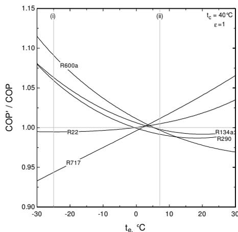
Figure 9. COP variation in case of constrained capacity for an IHX with  $\epsilon = 1$
