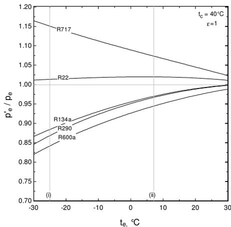
Figure 6. Evaporating pressure variation in case of constrained pressures for an IHX with  $\epsilon = 1$
