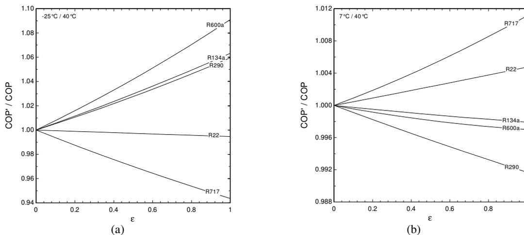
Figure 8. COP variation in case of constrained capacity: (a)  $t_e = -25^\circ\text{C}$  and (b)  $t_e = 7^\circ\text{C}$  ( $t_c = 40^\circ\text{C}$ )
