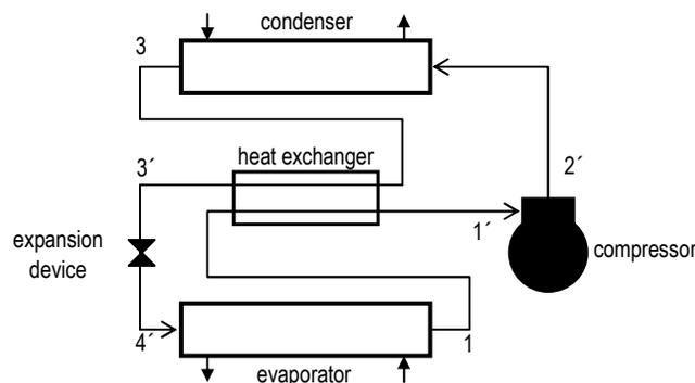
Figure 1. Schematic of the refrigeration cycle employing an internal heat exchanger
