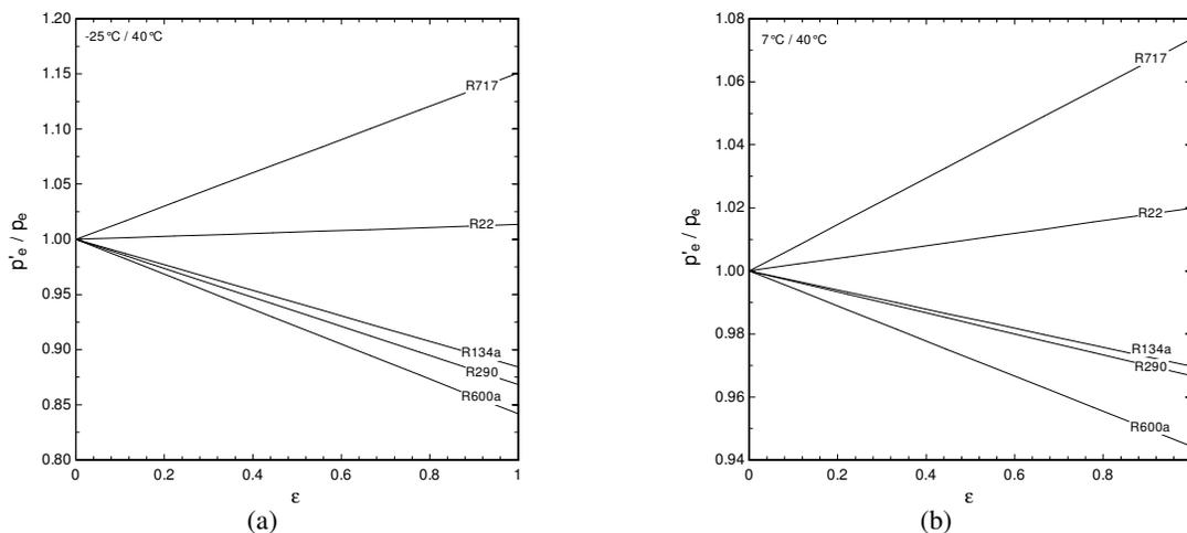
Figure 5. Evaporating pressure variation in case of constrained capacity: (a)  $t_c = -25^\circ\text{C}$  and (b)  $t_c = 7^\circ\text{C}$  ( $t_c = 40^\circ\text{C}$ )
