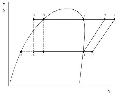
Figura 2. Thermodynamic representation of the refrigeration cycles under analysis in a p-h diagram
