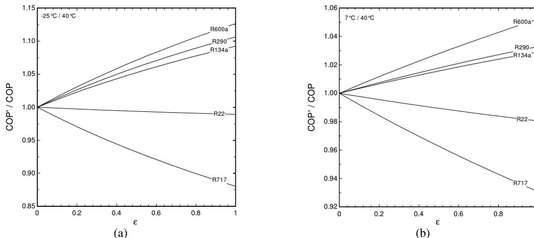
Figure 3. COP variation in case of constrained pressures: (a)  $t_e = -25^\circ\text{C}$  and (b)  $t_e = 7^\circ\text{C}$  ( $t_c = 40^\circ\text{C}$ )
