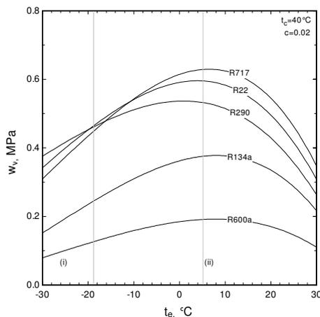
Figure 7. Mean effective pressure variation with the evaporating temperature
