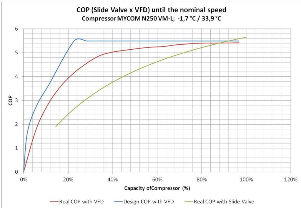
Figure 4. Comparison of COP and capacity in a screw compressor according type of control until 3550 rpm
