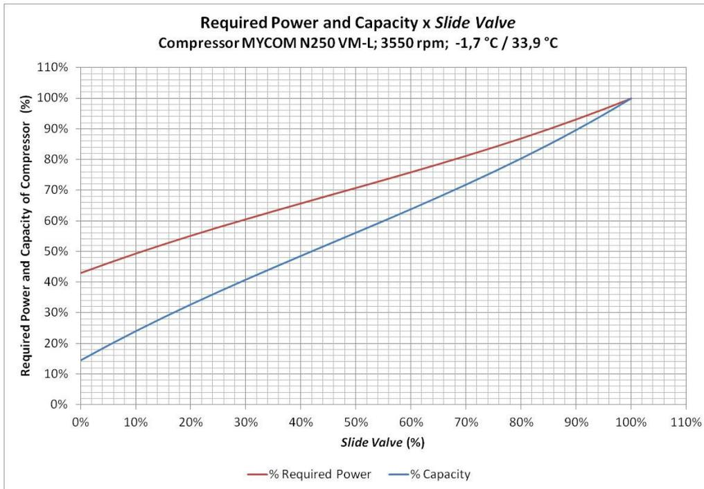
Figure 2. Required power and capacity of a compressor according to the opening of slide valve
