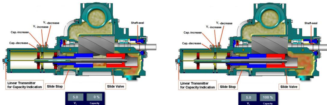
Figure 1. Operation of the slide valve (York Training and Developing DK, 2011)
