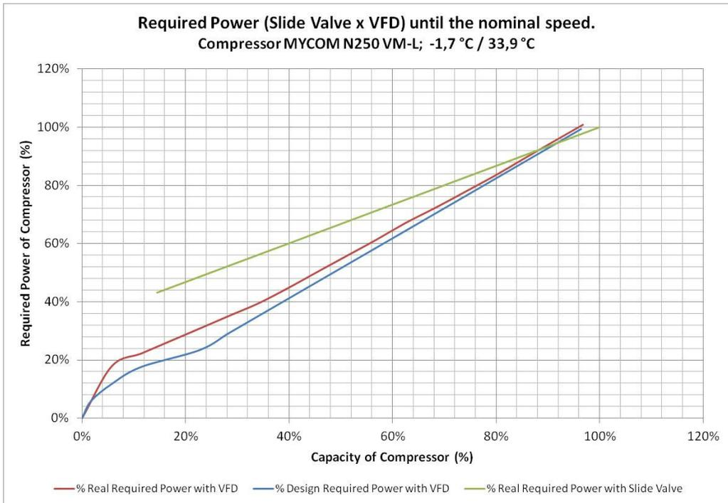
Figure 3. Comparison of required power and capacity in a screw compressor according type of control until 3550 rpm
