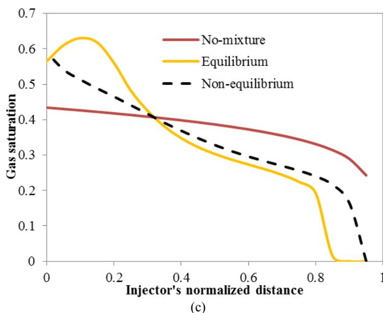
Figure 3. Gas saturation profile at 0.4 PV for injection rates of: a)  $1.71 \times 10^{-9} \text{ m}^3/\text{s}$ , b)  $1.71 \times 10^{-8} \text{ m}^3/\text{s}$ , and c)  $4.03 \times 10^{-8} \text{ m}^3/\text{s}$ .
