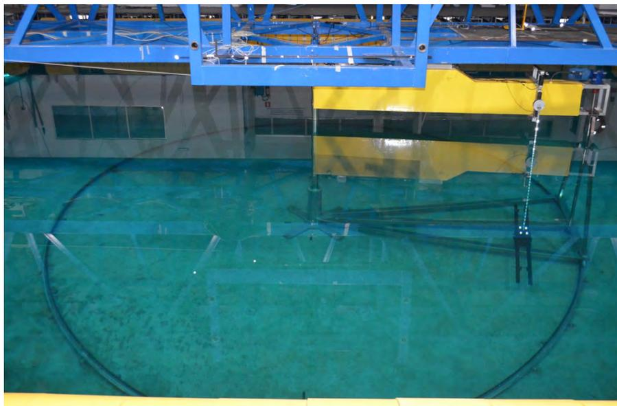
Figure 2. Rotating arm installed at Numerical Offshore Tank Hydrodynamic Calibrator.
