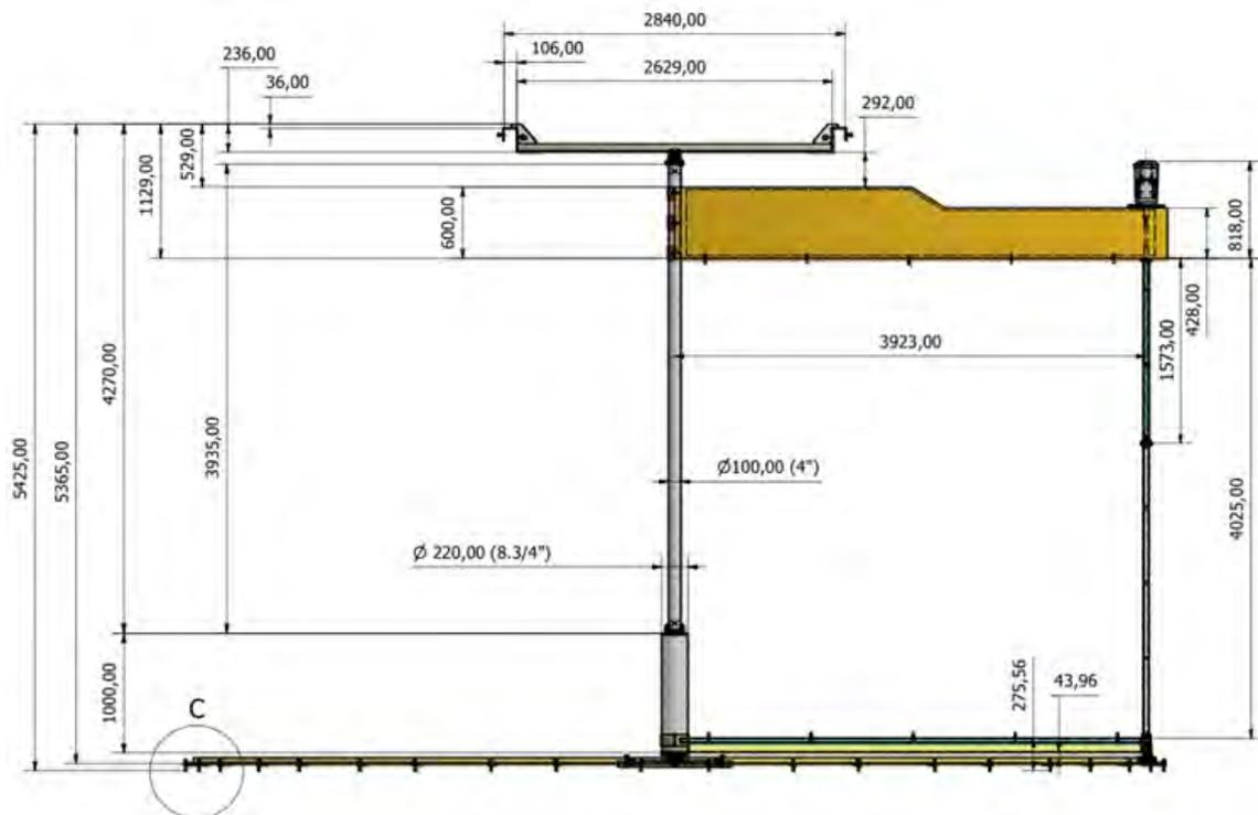
Figure 4. Rotating Arm Main Dimensions
