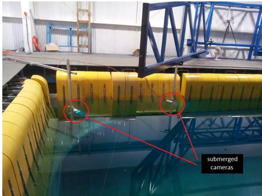
Figure 6. Two submerged cameras used to monitor the model tested in rotating arm.
