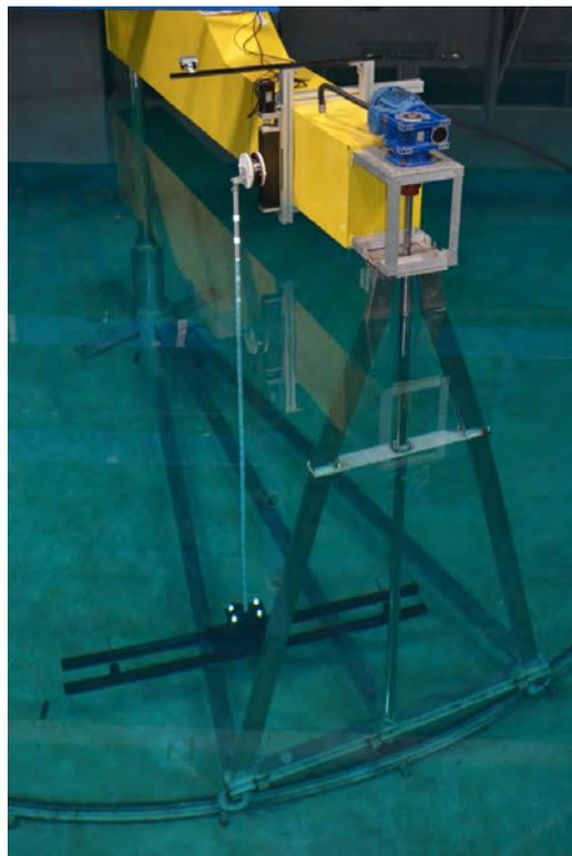
Figure 5. Approximate view of the rotating-arm equipped with a flexible line vertically arranged.
