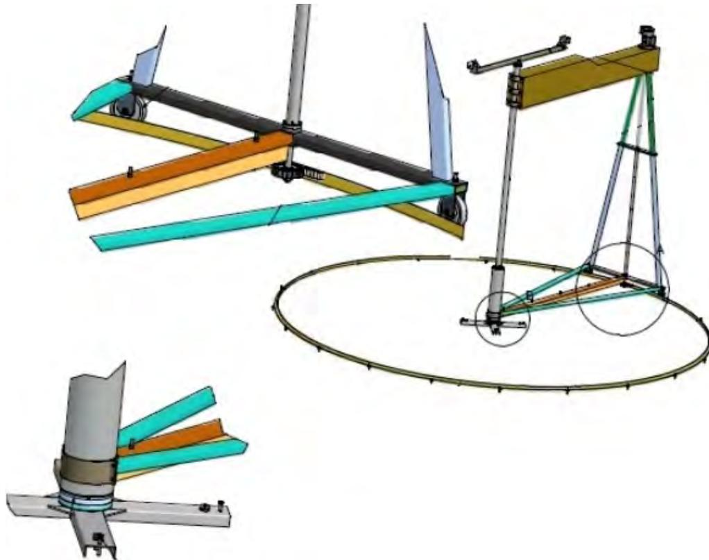
Figure 3. Schematic arrangement with details of the arm installed on the CH-TPN.
