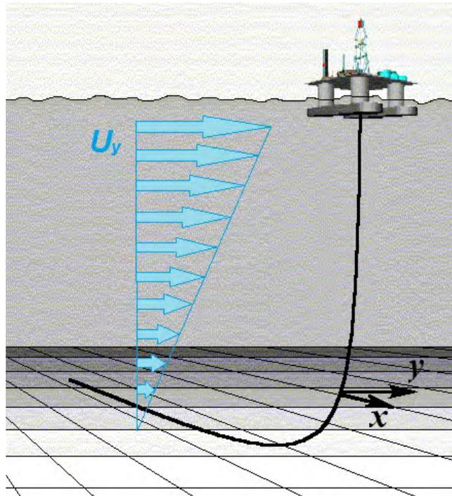
Figure 1. Schematic arrangement that illustrates the interesting problem: VIV acting on a riser.
