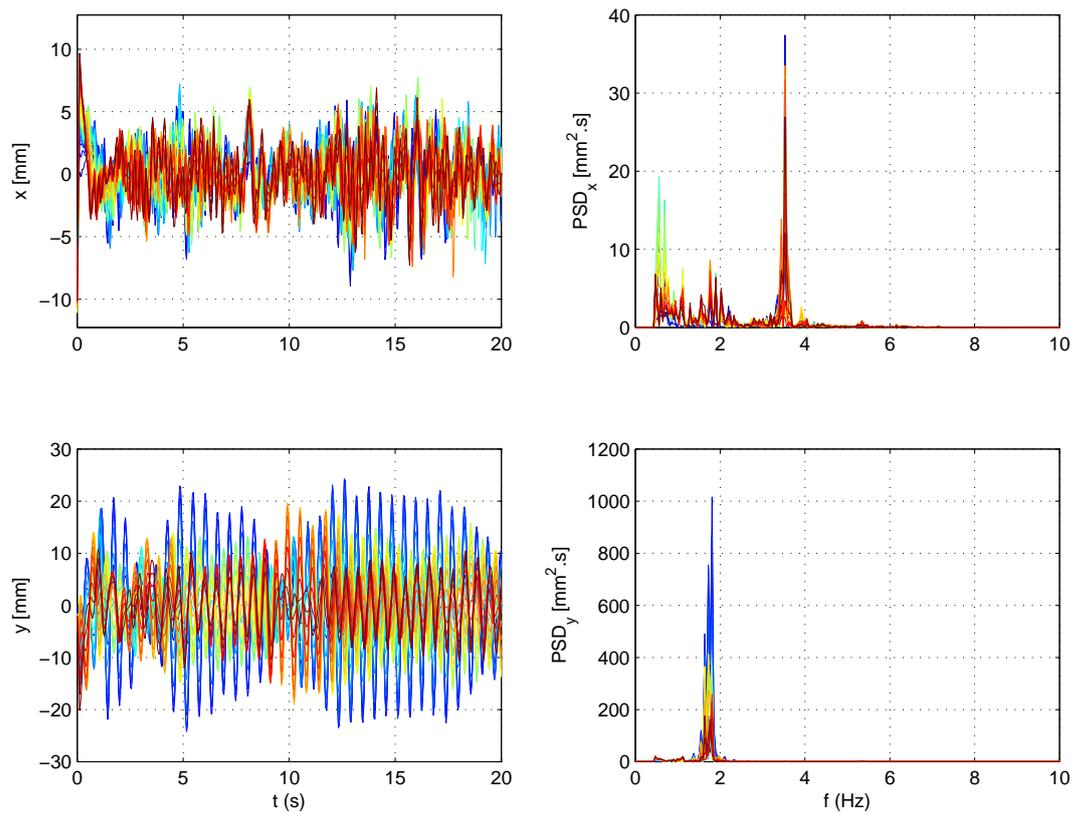
Figure 13. In-line and cross Power Density Spectrum of all obtained target trajectories.
