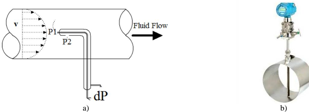
There are a lot of commercial Pitot tubes. Some equipment are more expensive and has data acquisition system that allows save or monitoring data in a computer, still there are cheaper ones whose data is shown in digital display (Fig. 1b).
