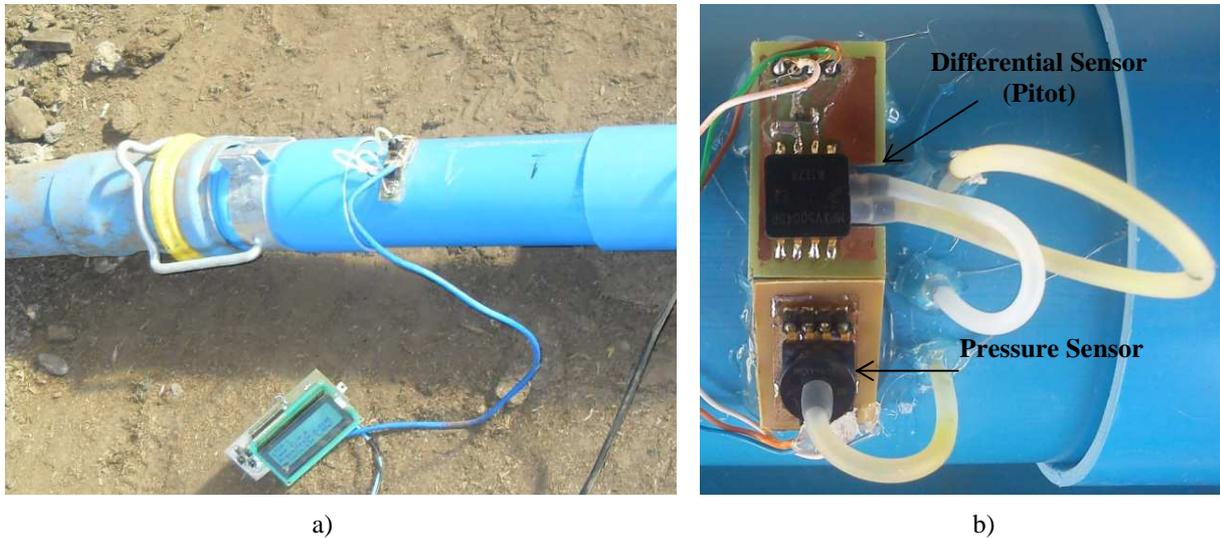
Figure 9. Details of the Pitot tube assembly in the pipelines. a) Device in operation and b) details of the assembly.
