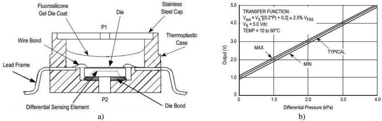
Figure 4. Details of sensors presented in Fig. 3c:
