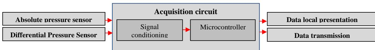
Figure 2. Block diagram of the system for measuring the pressure and air velocity
