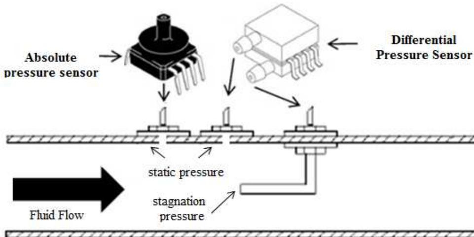
Figure 5. Schematic of the device developed for measuring air pressure and velocity. (Figueira Jr, 2012).
