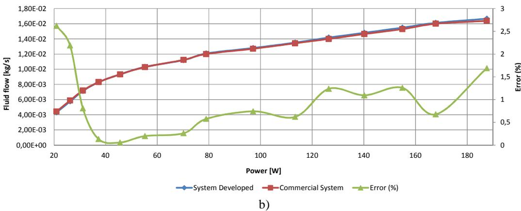
Figure 7. Data measured with the experimental device when compared with a commercial manometer: a) Pressure and b) Fluid flow.
