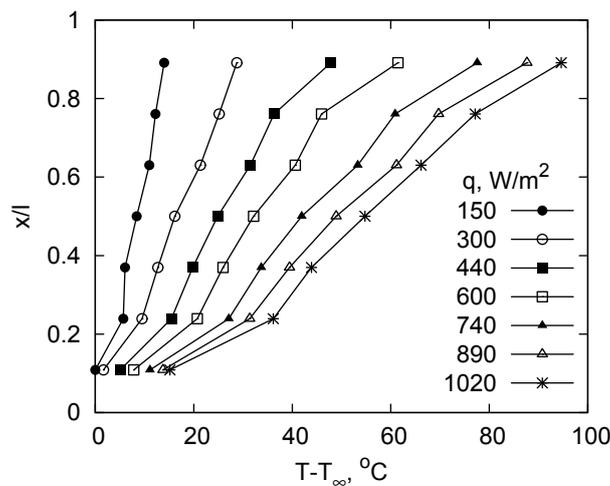
Figure 5. Measurements of the difference between the metallic wall temperature and the ambient temperature along the chimney height for several heat fluxes ( $l=2.3$  m). The connection between the points are only to facilitate visualization.
