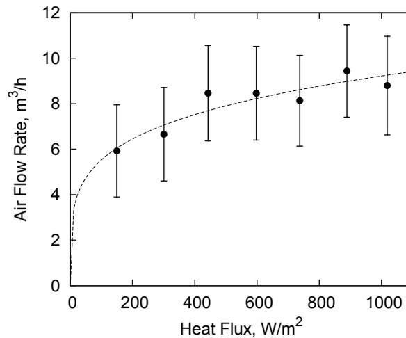
Figure 3. Volumetric flow rate through the solar chimney cavity for several inputs of heat fluxes, with error bars for the uncertainty and the fitted curve.
