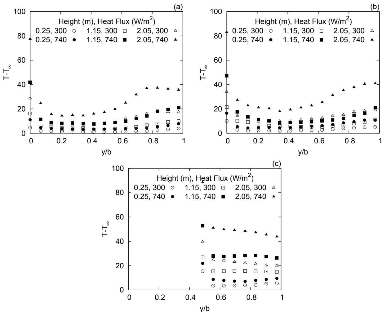
Figure 6. Difference between air temperature inside the chimney and the ambient air temperature, for some heights and two heat fluxes, from the hot to the isolated wall ( $b=36$  mm).
