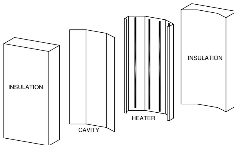
Figure 1. Main elements of the solar chimney.
