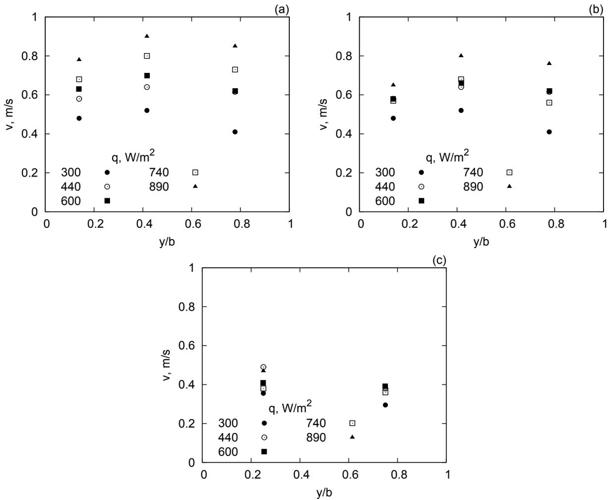
Figure 4. Air velocity from the metallic hot wall ( $y/l = 0$ ) to the isolated wall ( $y/l$ ), for  $z = 5$  mm (a),  $z = 15$  mm (b), and  $z = 70$  mm.
