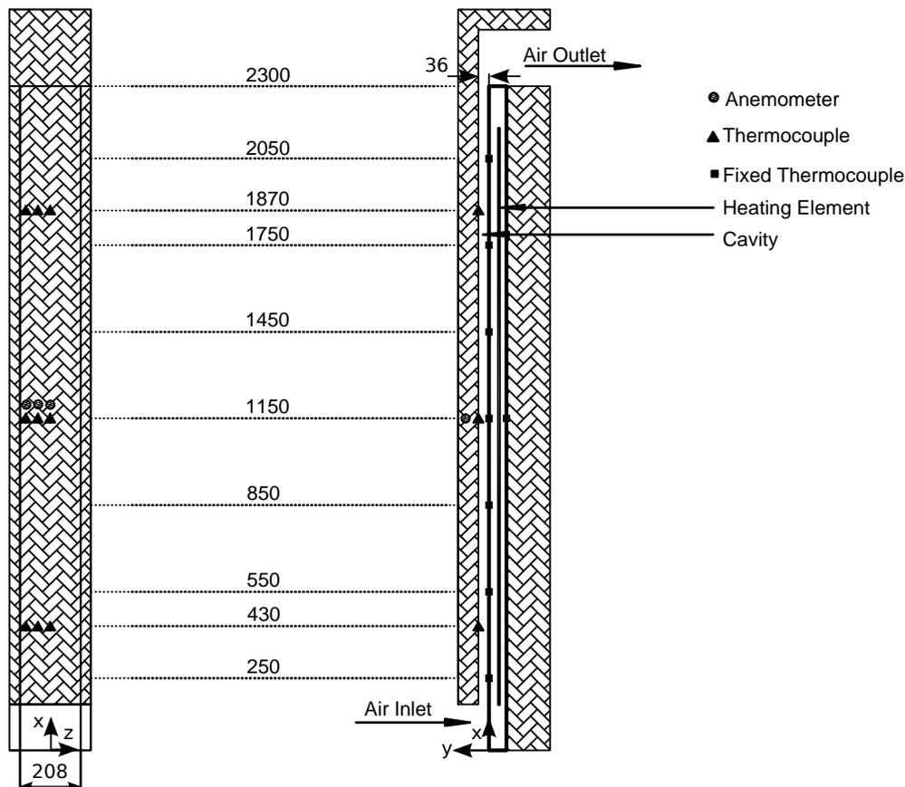
Figure 2. Experimental apparatus with the position of the sensors.
