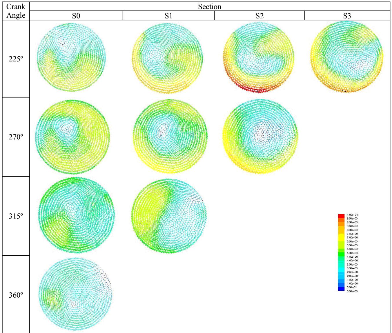
Figure 6. Swirl for the Otto cycle during compression stroke.
