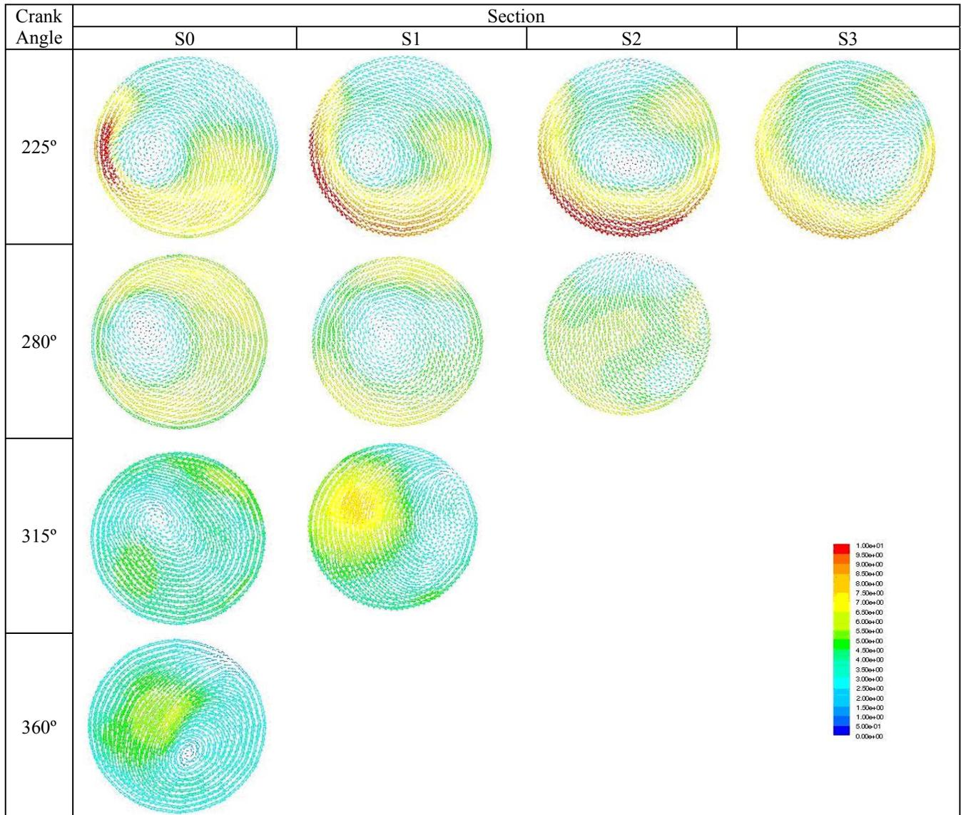
Figure 9. Swirl for the Miller LIVC cycle during compression stroke.
