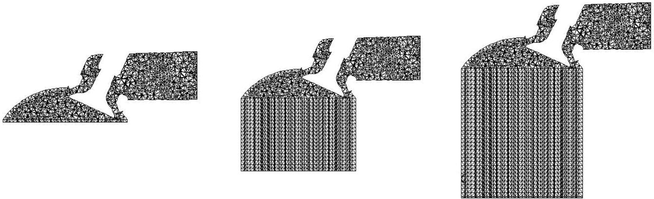
Figure 3. Mesh motion at 0°, 90°, 180°.
