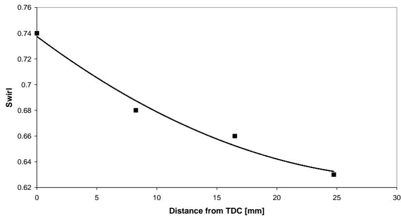
Figure 10. Evolution in swirl (2.5mm valve lift).
