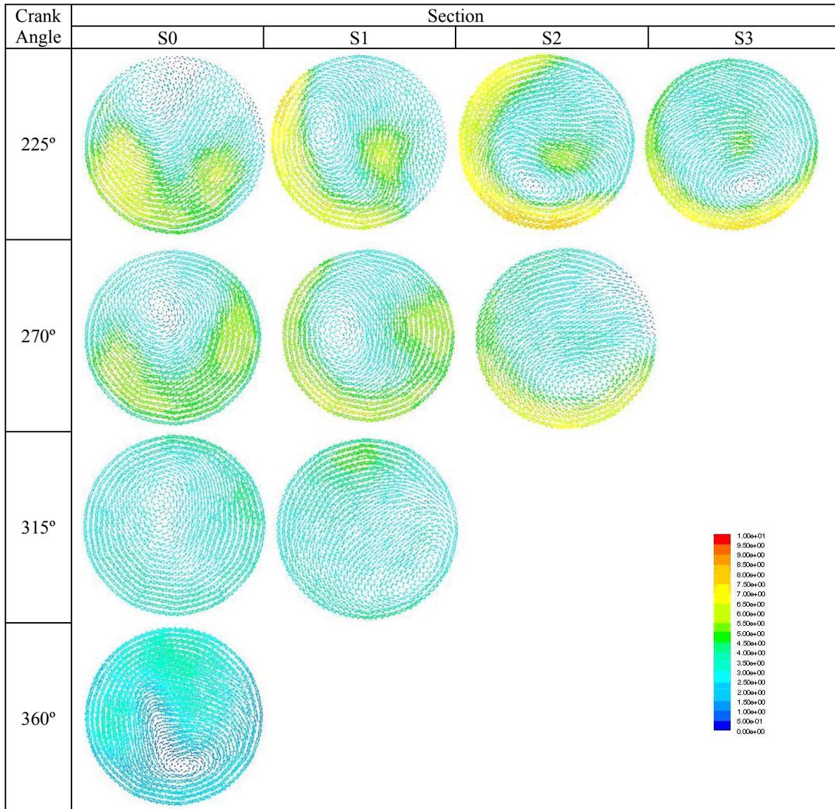
Figure 8. Swirl for the Miller EIVC cycle during compression stroke.
