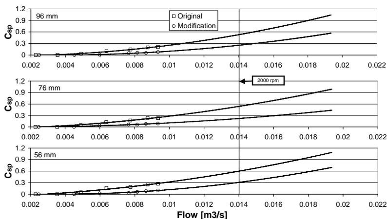
Figure 12. Swirl results after and before the intake duct modification.
