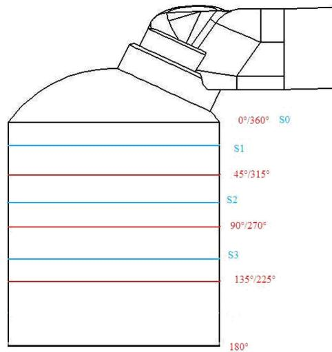
Figure 4. Cross sections for swirl measurement.
