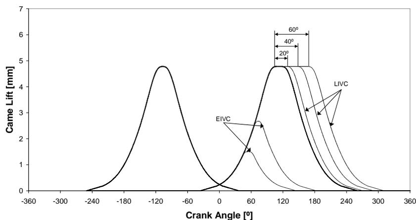
Figure 11. Different cam profiles tested.
