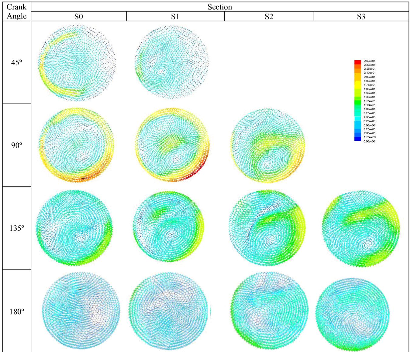
Figure 5. Swirl for the Otto cycle during intake stroke.
