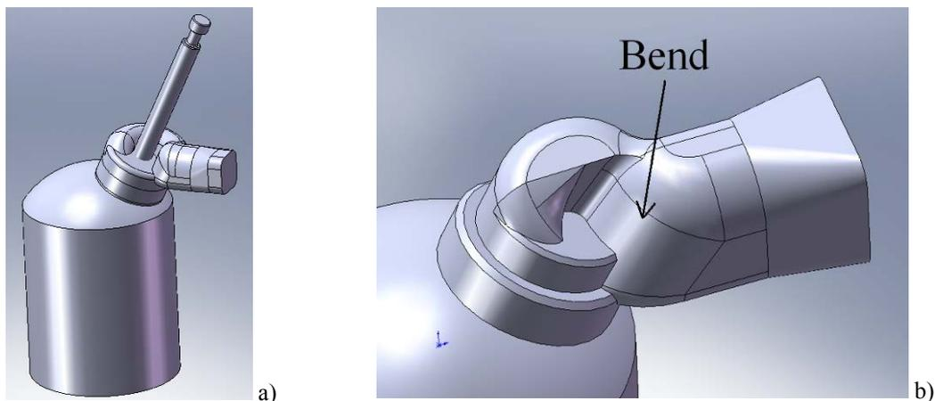
Figure 1. a)Design of intake port; b) Bend on the intake port.
