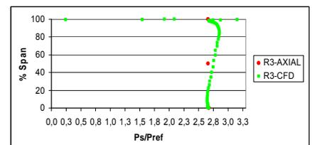
Figure 33. Static pressure distribution at the third rotor – AXIAL vs CFD.
