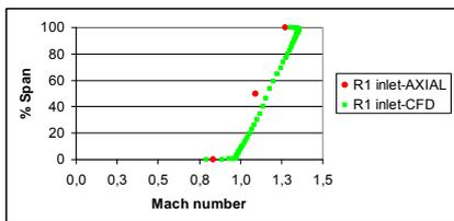
Figure 28. Mach number distribution at the first rotor – AXIAL vs CFD.
