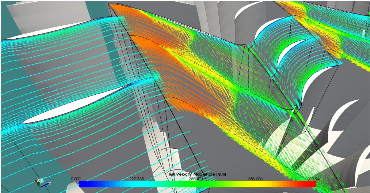
Figure 20. Velocity vectors close to compressor tip.
