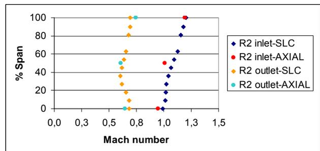
Figure 8. Comparison of the Mach number distribution at the second rotor.
