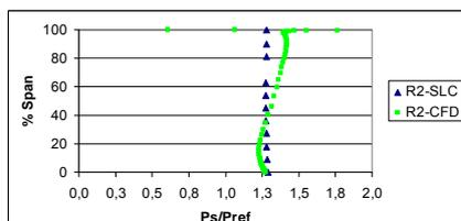
Figure 25. Static pressure distribution at second rotor – SLC vs CFD.
