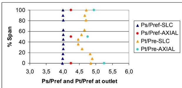
Figure 13. Static and total pressures distribution at the compressor outlet.
