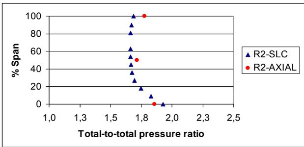
Figure 3. Comparison of the total-to-total pressure ratio at the second rotor.
