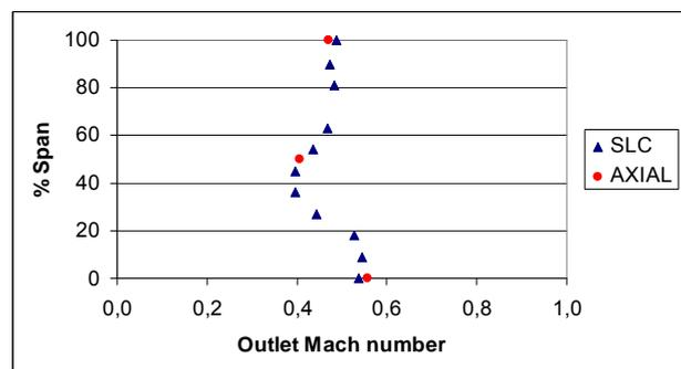
Figure 15. Mach number distribution at the compressor outlet.
