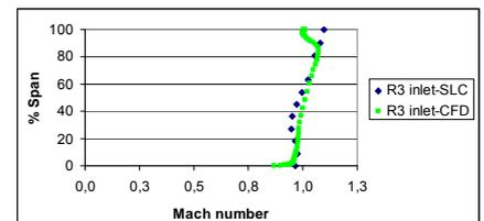
Figure 23. Mach number distribution at the third rotor – SLC vs CFD.
