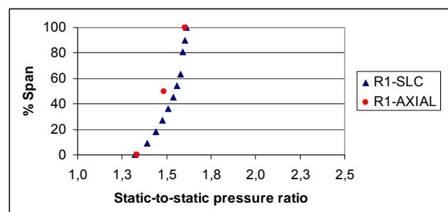
Figure 2. Comparison of the static-to-static pressure ratio at the first rotor.
