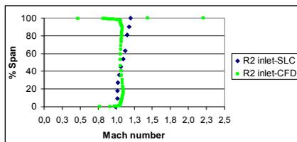
Figure 22. Mach number distribution at the second rotor – SLC vs CFD.
