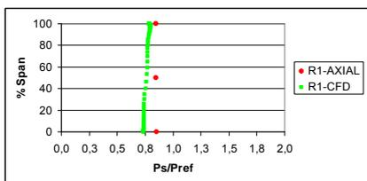
Figure 31. Static pressure distribution at the first rotor – AXIAL vs CFD.
