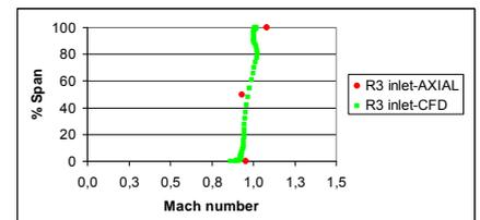
Figure 30. Mach number distribution at the third rotor – AXIAL vs CFD.
