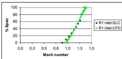
Figure 21. Mach number distribution at the first rotor – SLC vs CFD.
