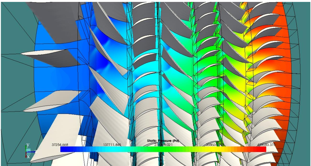
Figure 19. Static pressure contours at the compressor mean diameter.
