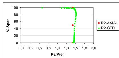
Figure 32. Static pressure distribution at the second rotor – AXIAL vs CFD.
