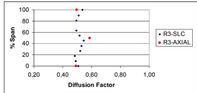
Figure 12. Diffusion factor distribution at the third rotor along the blade height.
