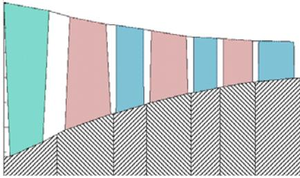
Figure 16. Meridional view of the compressor.
