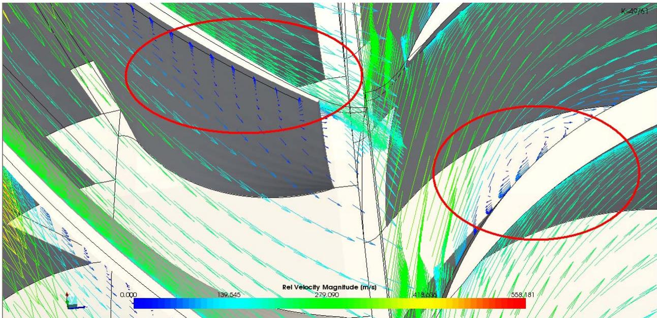
Figure 27. Velocity vectors at the compressor mean diameter.
