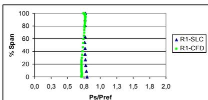
Figure 24. Static pressure distribution at first rotor – SLC vs CFD.
