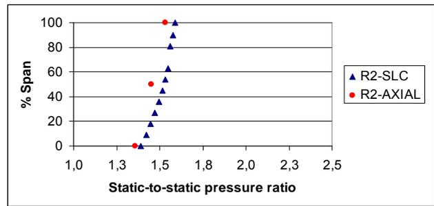
Figure 3. Comparison of the static-to-static pressure ratio at the second rotor.
