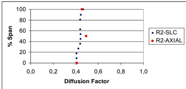
Figure 11. Diffusion factor distribution at the second rotor along the blade height.
