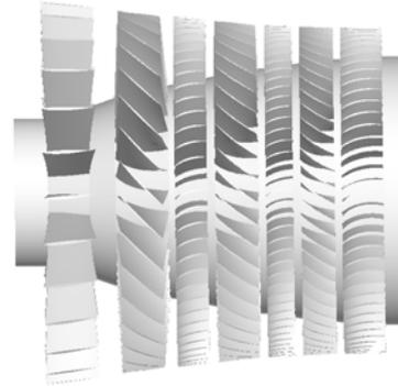
Figure 17. 3D view of the blade profiles.
