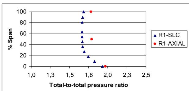
Figure 1. Comparison of the total-to-total pressure ratio at the first rotor.
