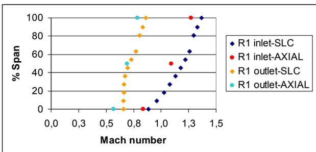
Figure 7. Comparison of the Mach number distribution at the first rotor.
