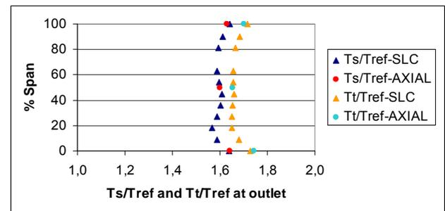
Figure 14. Static and total temperatures distribution at the compressor outlet.
