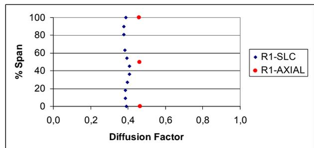
Figure 10. Diffusion factor distribution at the first rotor along the blade height.
