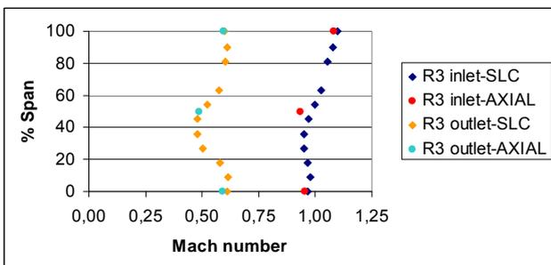
Figure 9. Comparison of the Mach number distribution at the third rotor.
