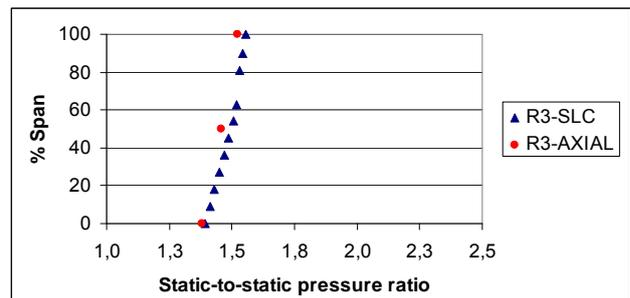
Figure 6. Comparison of the static-to-static pressure ratio at the third rotor.
