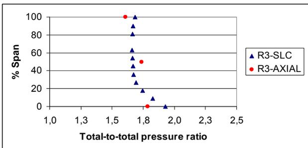
Figure 5. Comparison of the total-to-total pressure ratio at the third rotor.
