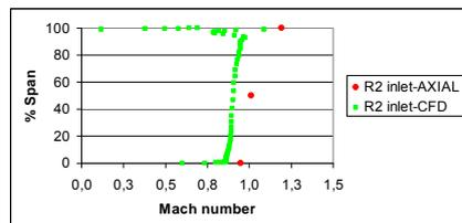
Figure 29. Mach number distribution at the second rotor – AXIAL vs CFD.
