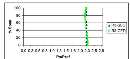
Figure 26. Static pressure distribution at third rotor – SLC vs CFD.
