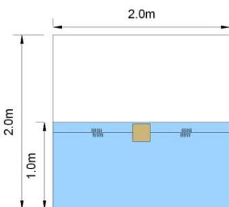
Figure 13 – Dimensions of the model used to compare results of sloshing with a submerged body.
