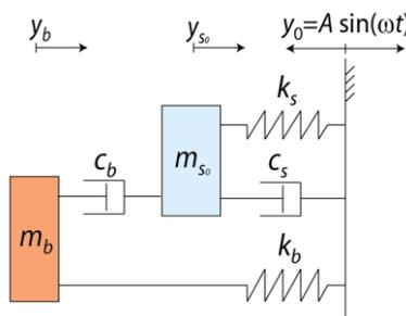
Figure 10 – Rearranged diagram of the mass-spring-damping system of the model.
