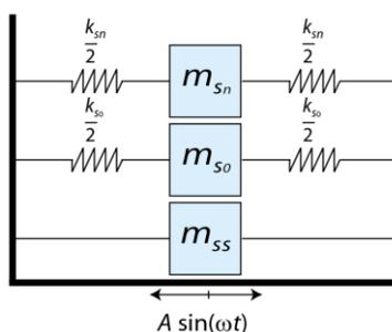
Figure 5 – Mechanical system diagram representing sloshing
