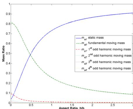
Figure 7 – Masses for sloshing mechanical system
