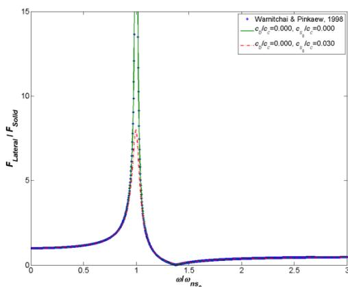
Figure 12 – Lateral forces due to sloshing as a function of the period of excitation of a tank with a width of 2.0m of water level of completion of 1.0m.
