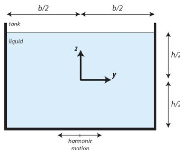
Figure 3 – Coordinate system and geometry of the rectangular tank
