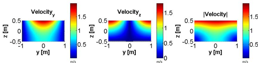
Figure 4 – y and z components and the absolute values of the velocity amplitude of the liquid in a tank with width of 1.0 m and filling level of 1.0 m and excitation amplitude of 1.0cm.
