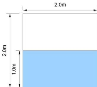
Figure 11 – Dimensions of the model used to compare results of sloshing.
