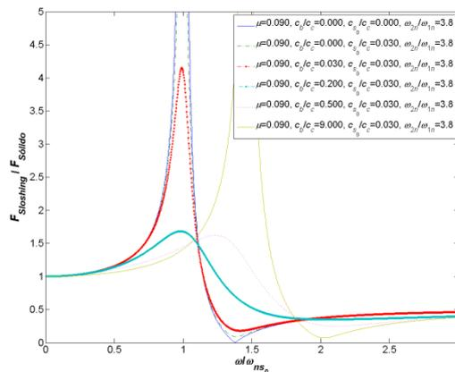
Figure 14 – Lateral forces due to sloshing depending on the period of excitation of a tank with a width of 2.0 m of fill level of 1.0 m of water with a submerged body.
