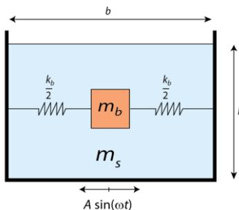
Figure 8 – Rectangular tank filled partially with a submerged body connected by horizontal springs.
