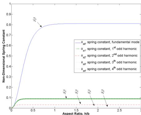
Figure 6 – Spring constants for sloshing mechanical system
