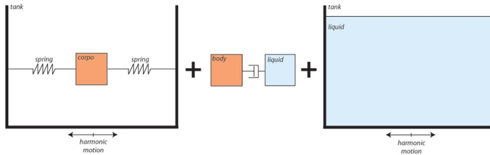
Figure 2 – Damping force used to connect two mechanical systems.
