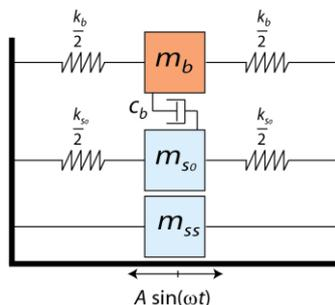
Figure 9 – Diagram of the mass-spring-damping system of the model.
