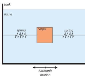
Figure 1 – Tank partially filled with liquid and a submerged body connected elastically to the tank.
