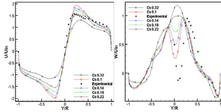
Figure 2: Radial profiles of the average velocities, tangential (left), axial (right), for different Smagorinsky constants, from top to bottom  $Z/D = 0.89, 1.39, 1.89$  and  $2.39$ .
