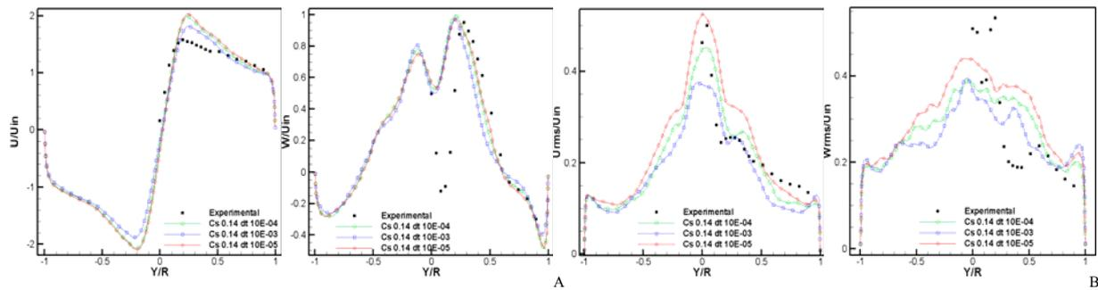
Figure 5: Radial profiles of the average velocities, tangential (left), axial (right), for different time steps, from top to bottom  $Z/D = 0.89, 1.39, 1.89$  and  $2.39$  (A). Radial profiles of the average RMS velocities, tangential (left), axial (right), for different time steps, from top to bottom  $Z/D = 0.89, 1.39, 1.89$  and  $2.39$  (B).
