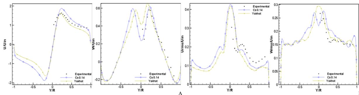
Figure 7: Radial profiles of the average velocities, tangential (left), axial (right), for different turbulence models,  $Z/D = 1.39$  (A). Radial profiles of the average RMS velocities, tangential (left), axial (right), for different turbulence models,  $Z/D = 1.39$  (B).
