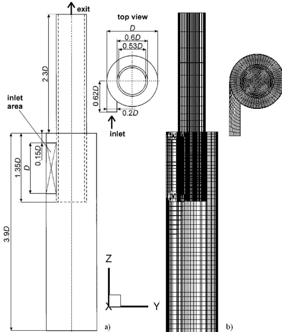
Figure 1: a - Flow geometry (adapted from Derksen and Van den Akker, 2000). b- Computational grid.
