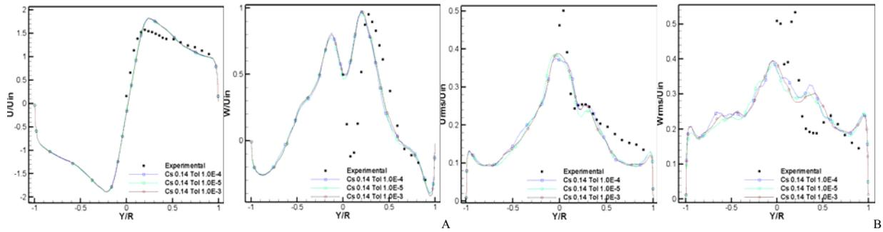
Figure 4: Radial profiles of the average velocities, tangential (left), axial (right), for different solver tolerance, from top to bottom  $Z/D = 0.89, 1.39, 1.89$  and  $2.39$  (A). Radial profiles of the average RMS velocities, tangential (left), axial (right), for different solver tolerance, from top to bottom  $Z/D = 0.89, 1.39, 1.89$  and  $2.39$  (B).
