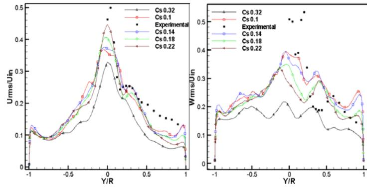
Figure 3: Radial profiles of the average RMS velocities, tangential (left), axial (right), for different Smagorinsky constants, from top to bottom  $Z/D = 0.89, 1.39, 1.89$  and  $2.39$ .
