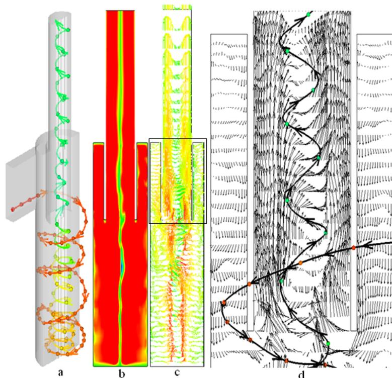
Figure 6: Details of the average (a) and instantaneous (b, c and d) flow field inside the cyclone.
