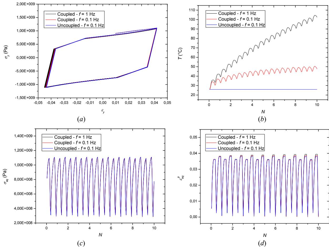
Figure 11. Stress-strain curve (a). Temperature (b), *von Mises* equivalent stress (c) and equivalent plastic strain (d) evolution.
