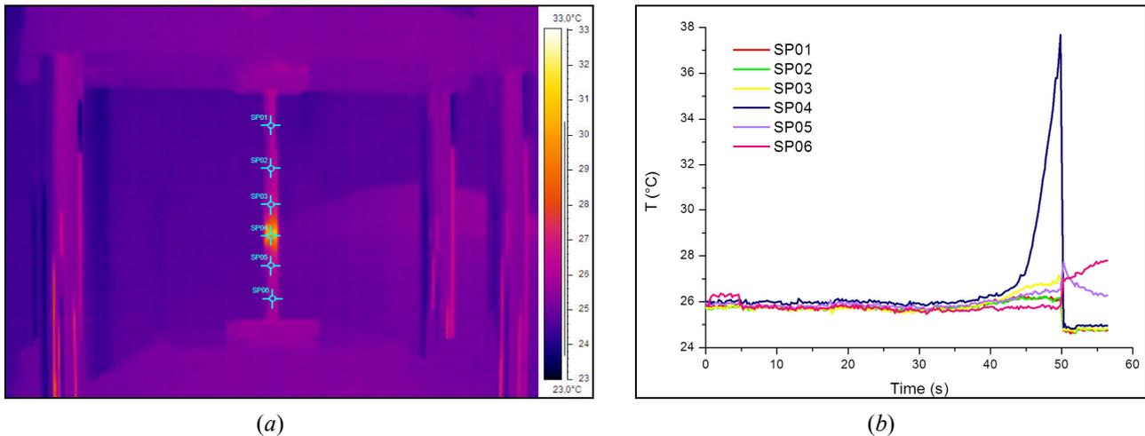
Figure 2. Thermal data from a tensile test: (a) infrared (IR) thermal image and (b) temperature evolution at 6 positions.
