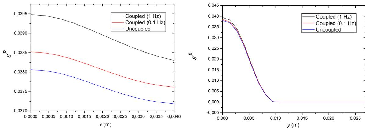
Figure 10. Plastic strain and temperature distribution through  $x$  and  $y$  axis. *Uncoupled and coupled models*.
