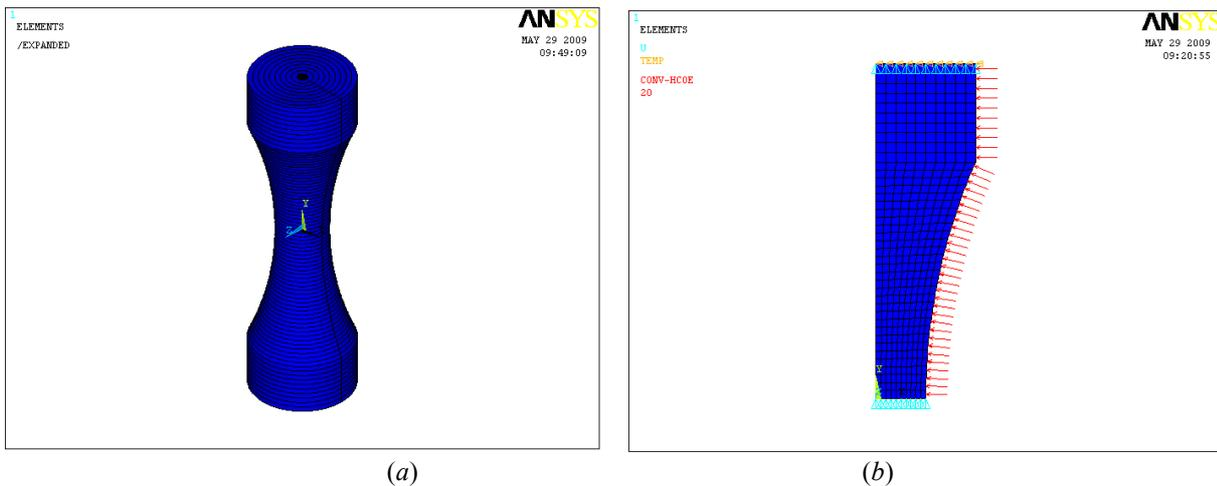
Figure 5. Hour-glass fatigue test specimen (a) and axisymmetric mesh with boundary conditions and loadings (b).
