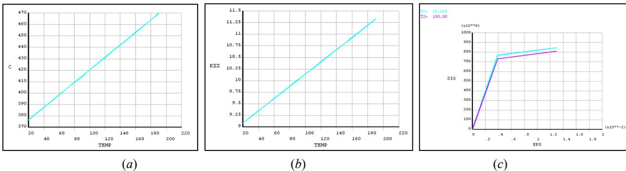
Figure 6. AISI 4140 temperature dependent thermomechanical properties: (a) specific heat, (b) thermal conductivity and (c) stress-strain curve.
