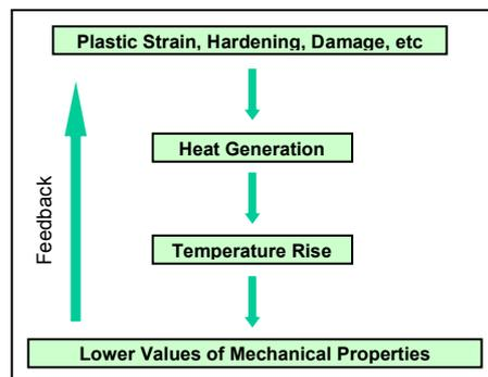
Figure 1. Thermomechanical coupling in metallic elements subjected to inelastic strain loadings.
