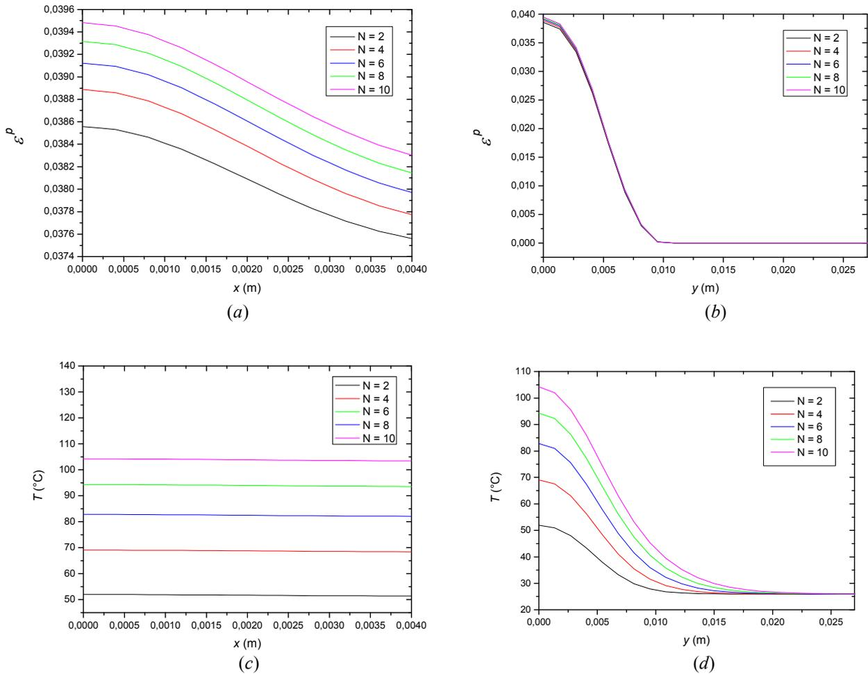
Figure 9. Plastic strain and temperature distribution through  $x$  and  $y$  axis. *Coupled model* for 1 Hz.
