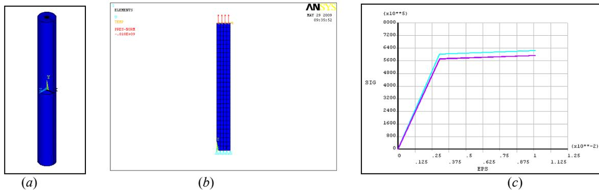
Figure 3. Tensile test specimen geometry (a), boundary conditions and mechanical loading (b) and material stress-strain curve (c).
