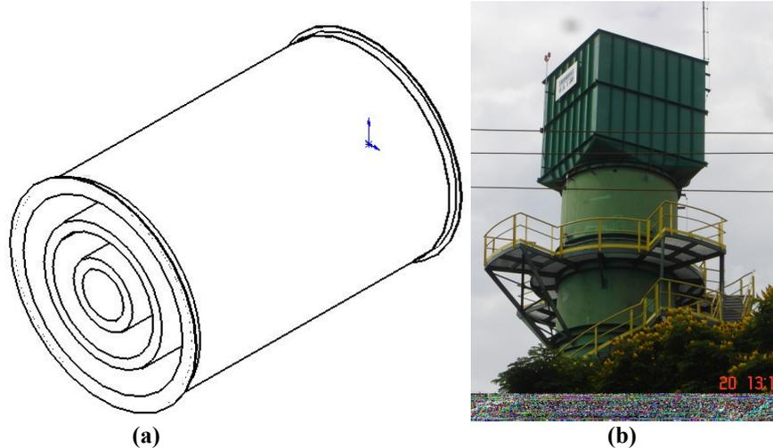
**Figure 2.1 – Baffle-type dissipative silencer: a) with concentric baffles; b) with rectangular baffles.**
