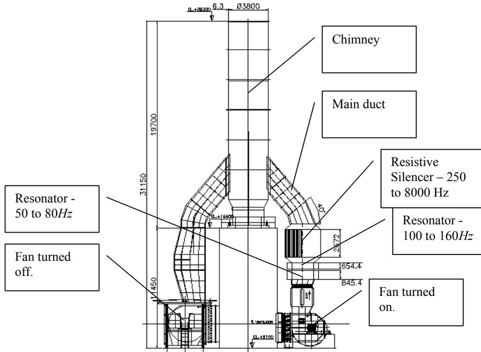
Figura 6.1 – Exhaustion system with optimum noise control system.
