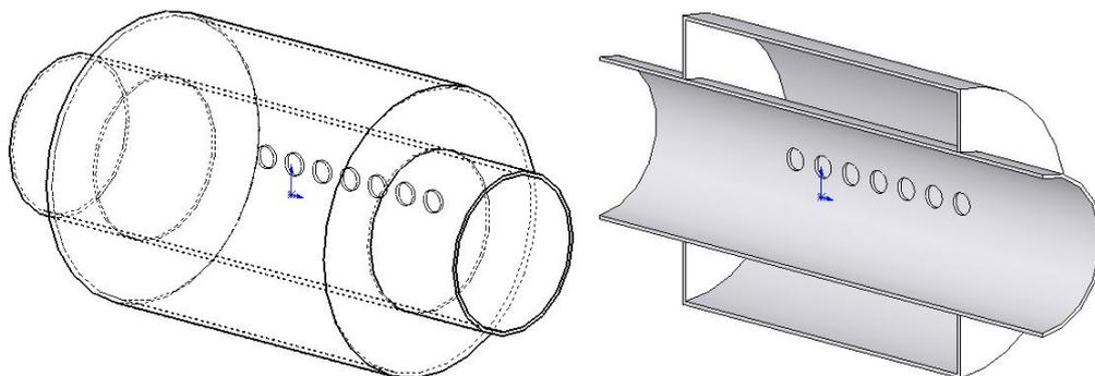
**Figure 3.1 – Side-branch resonator.**
