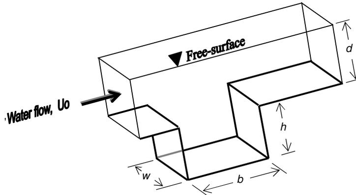
Figure 1: Open cavity geometric parameters.
