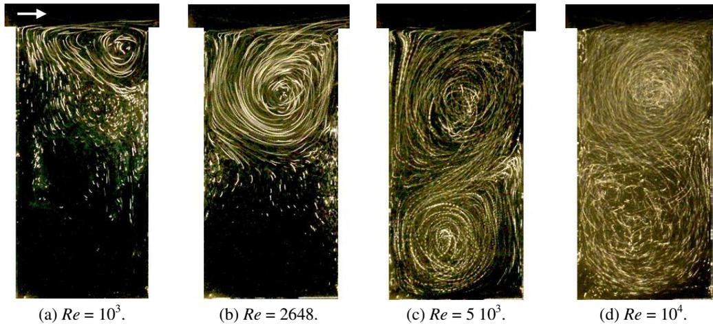
Figure 7: Flow visualization inside a cavity with  $b/h = 0.5$  provided with the help of solid tracers.
