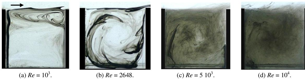
Figure 5: Flow visualization inside a cavity with  $b/h = 1$  provided with the help of liquid dye injection.
