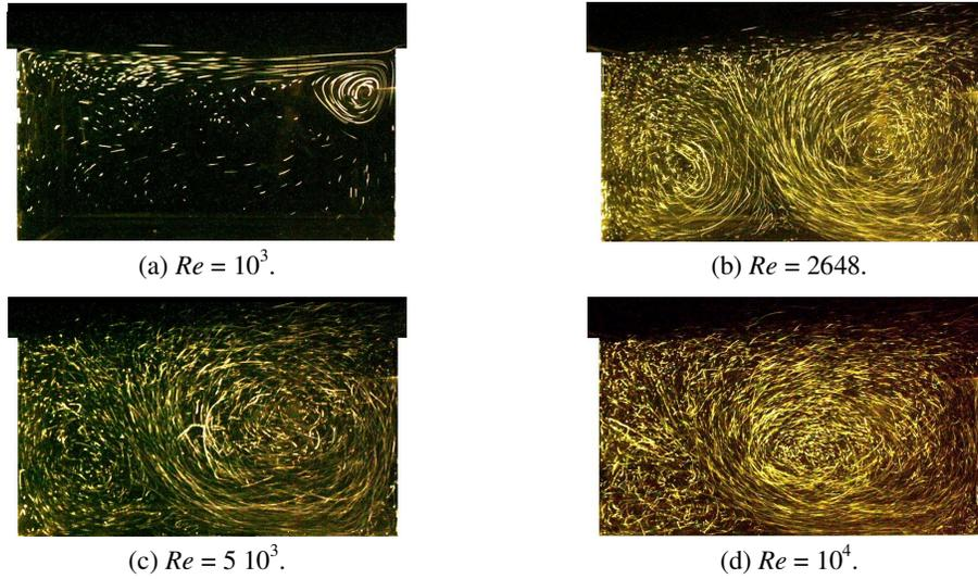
Figure 9: Flow visualization inside a cavity with  $b/h = 2$  provided with the help of solid tracers.
