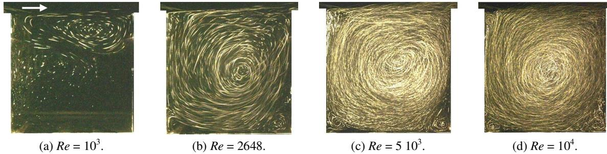
Figure 4: Flow visualization inside a cavity with  $b/h = 1$  provided with the help of solid tracers.
