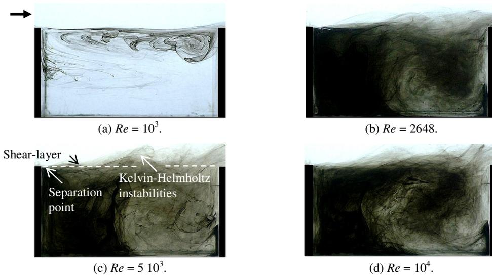
Figure 10: Flow visualization inside a cavity with  $b/h = 2$  provided with the help of liquid dye injection.
