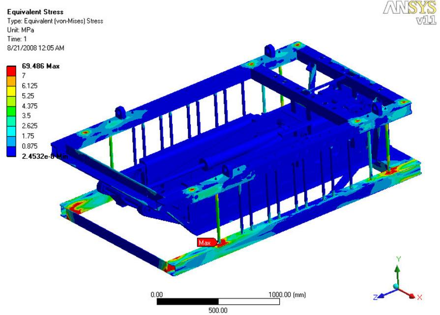
Figure 8. Von-Mises stresses due to landing.
