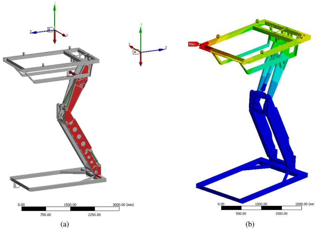
Figure 9. Limit configuration at working configuration. (a) Load conditions. (b) Deformations.
