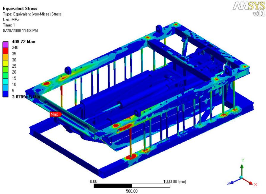
Figure 7. BUPPA stresses due to ROV installation.
