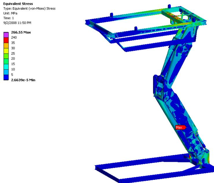
Figure 10. Von-Mises Stresses for collision simulation.
