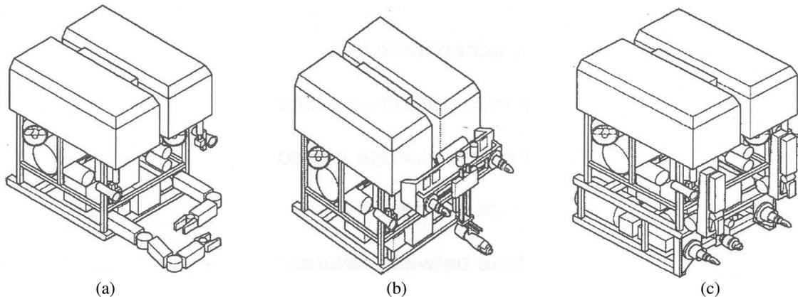
Figure 2. ROV intervention tasks configurations: (a) with manipulators. (b) with twin-point docking tool (TDU). (c) with underslung tool skid. (ISO, 2002).
