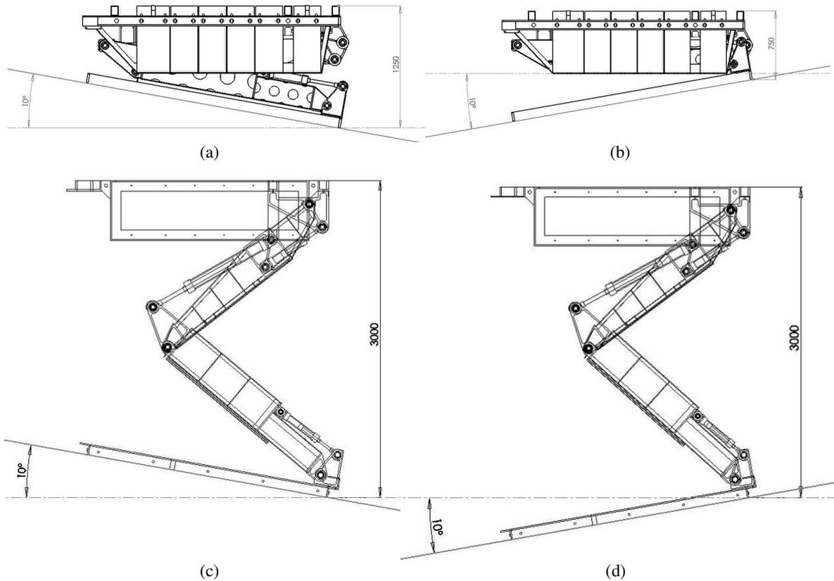
Figure 4: BUPPA limit configurations. (a) and (b) lower positions. (c) and (d) upper positions.
