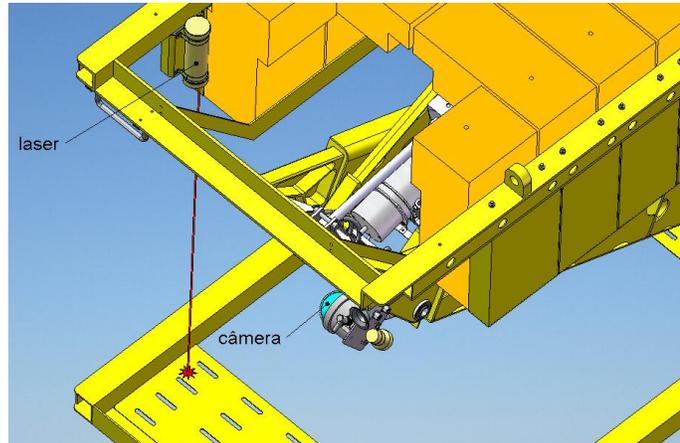
Figure 5: Monitored action for lifting motion.
