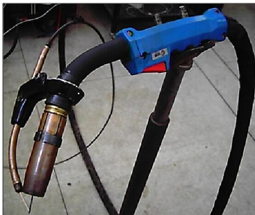
Figure 1. Welding torch connected to the feed device of the cold wire.
