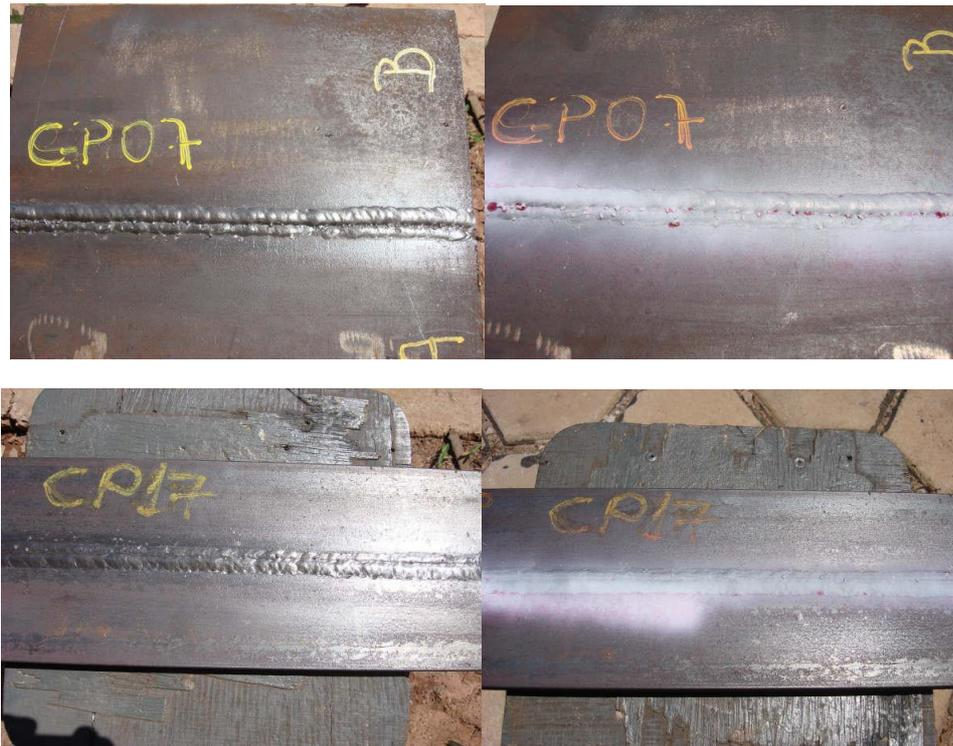
Figure 3. Superficial aspect of the welded joints by FCAW-CW welding process (CP07), and FCAW welding process (CP 17).
