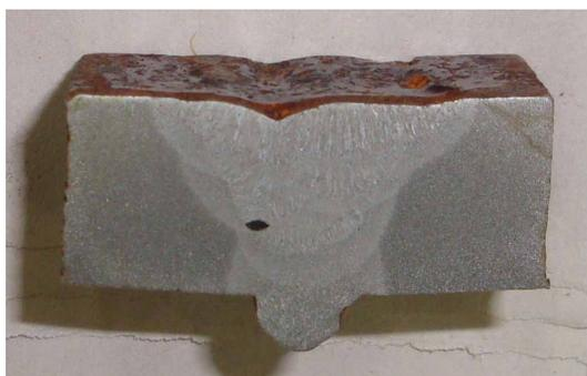
Figure 5. FCAW cross sectional macrography. The surface was etched by Nital 2%, zoom 1,5x.
