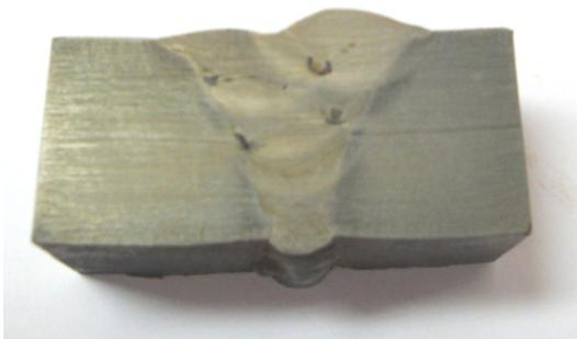
Figure 4. FCAW-CW cross sectional macrography. Etched surface by Nital 2%, zoom 1,5x.
