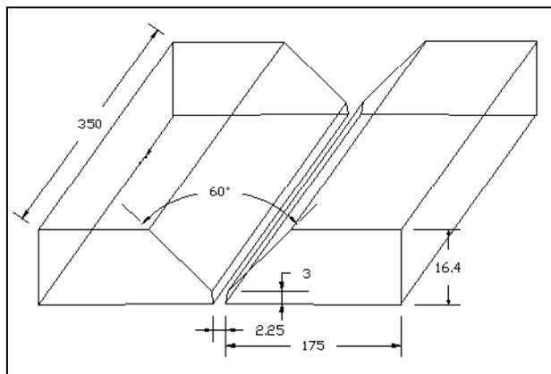
Figure 2. Details of the joint construction.
