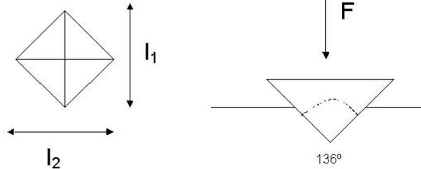
Where  $F$  is the load in grams and  $l_1$  and  $l_2$  are the lengths of the diagonals left by the indenter as shown in Figure 3. Figure 4 shows the Vickers hardness setup.
