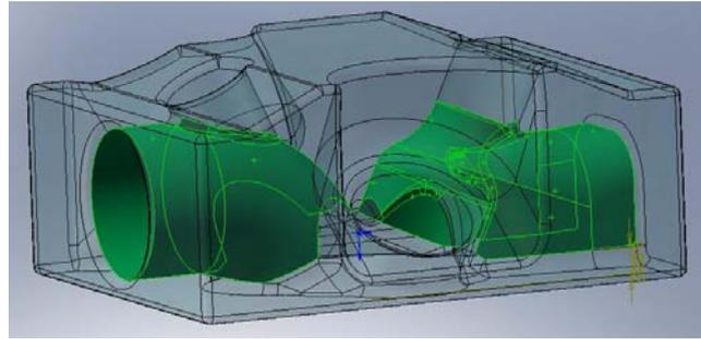
Figure 8. Coolant chamber with inlet (right) and exhaust (left) ports highlighted
