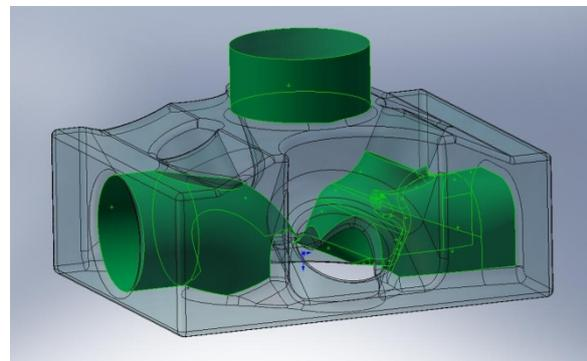
Figure 9. Design #2 - Half cut cylinder head (left) and coolant chamber (right)
