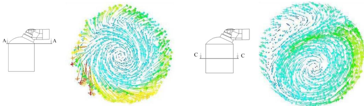
Figure 6. Final geometry with FLUENT (swirl) results at two locations of the cylinder
