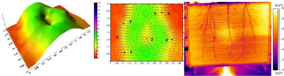
Figure 10. Air velocity profile and surface temperature – Fan with converger operating with frontal wind of 30km/h.
