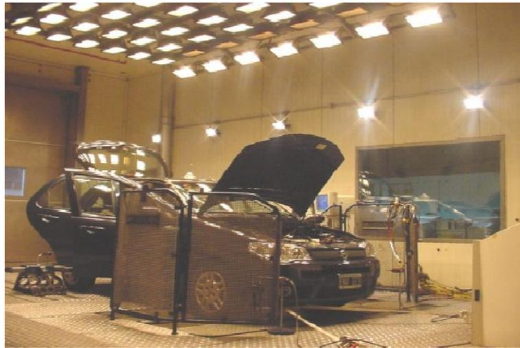
Figure 1. Climatic chamber with a roller dynamometer (Fiat Automóveis S.A.,2008)
