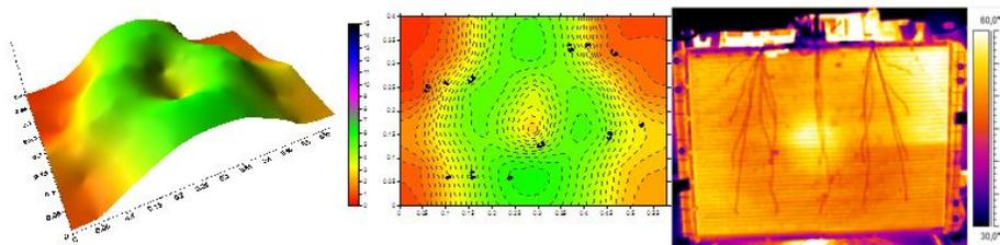
Figure 11. Perfil Air velocity profile and surface temperature – Fan without converger operating with frontal wind of 30km/h.
