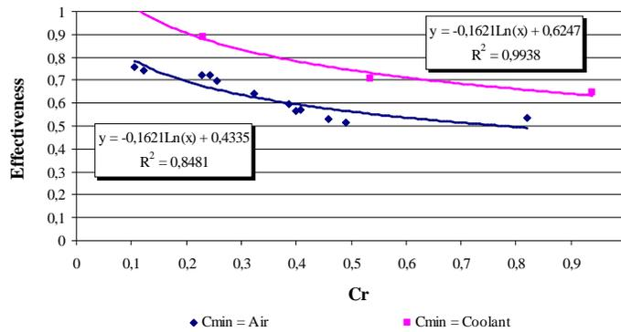
Figure 6. Effectiveness as a function of capacity rate ratio.
