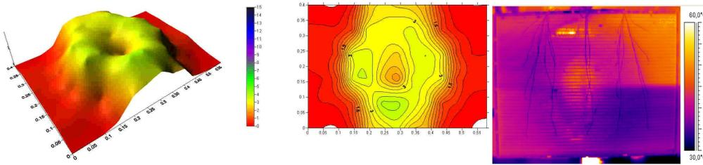
Figure 9 – Air velocity profile and surface temperature - Fan without converger operating without frontal wind
