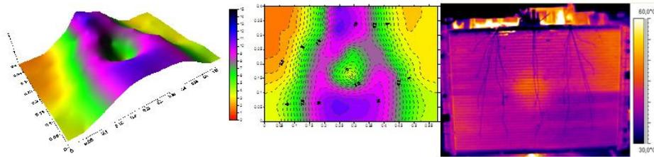
Figura 13. Perfil Perfil Air velocity profile and surface temperature – Fan without converger operating with frontal wind of 72 km/h
