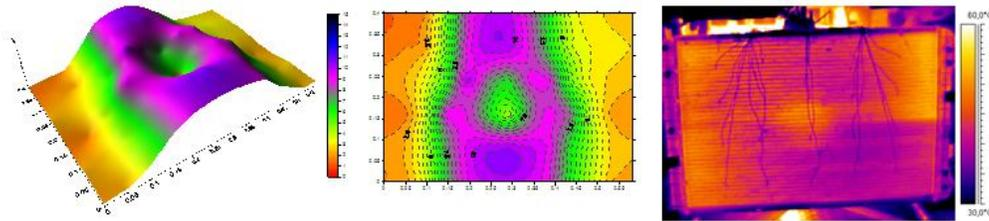
Figura 12. Air velocity profile and surface temperature – Fan with converger operating with frontal wind of 72 km/h
