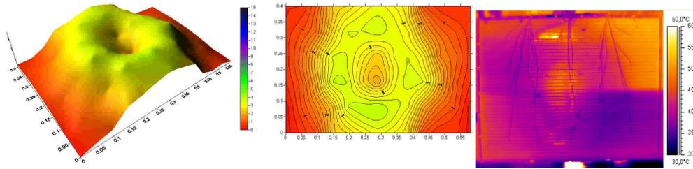
Figure 8 – Air velocity profile and surface temperature – Fan with converger operating without frontal wind.
