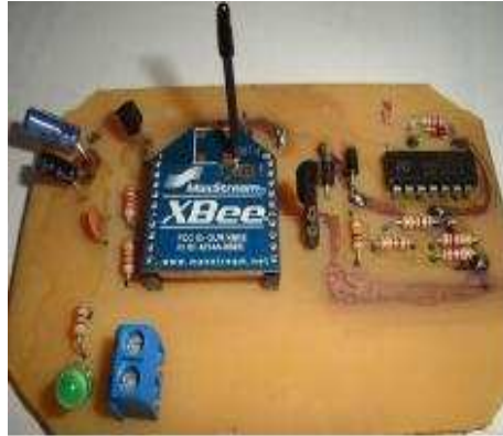
Figure 4. Diagram of the End Device Sensor (Filho and Dias, 2008).
