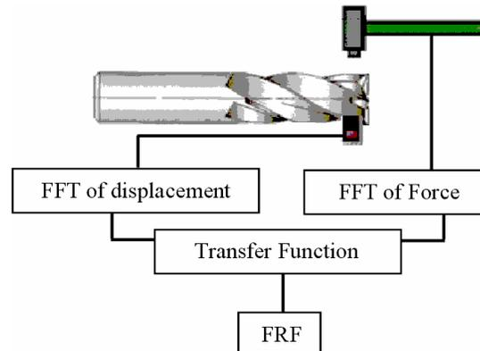
Figure 3. Procedure to obtain the FRF of the assembly.
