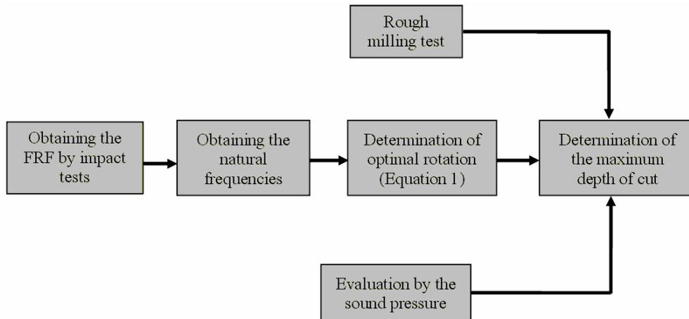
Figure 2. Flowchart to determine the optimal parameters.
