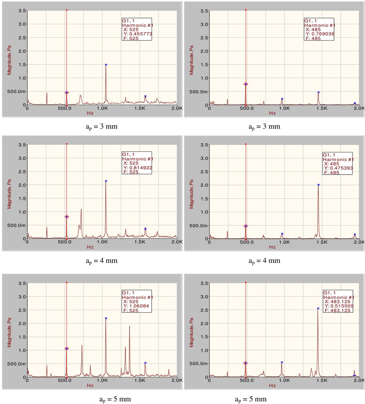
Figure 8. Sound spectrum – (G1;1: Average auto power spectrum and F: frequency of passages of teeth).
