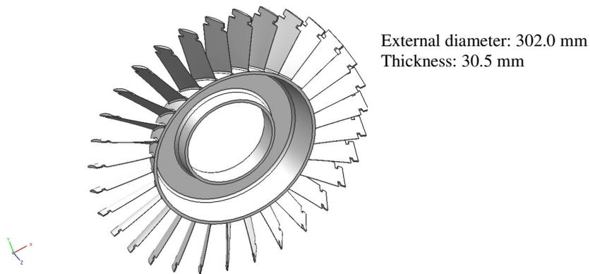
Figure 1. Aluminum stator.
