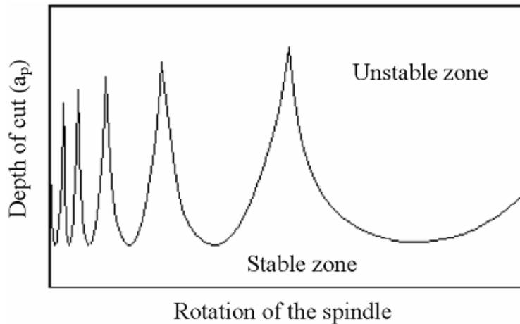
Figure 4. Example of stability lobe diagram.
