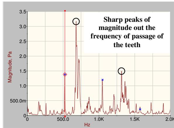
Figure 9. A Condition:  $n = 15,750$  rpm,  $a_p = 6$  mm.
