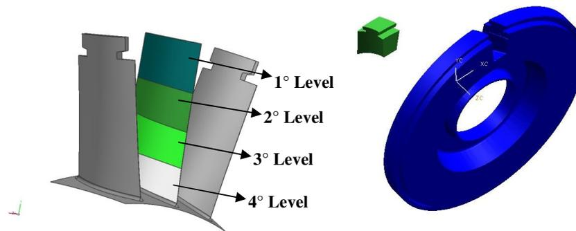
Figure 7. Levels of the region machined and unit volume removed between the blades.
