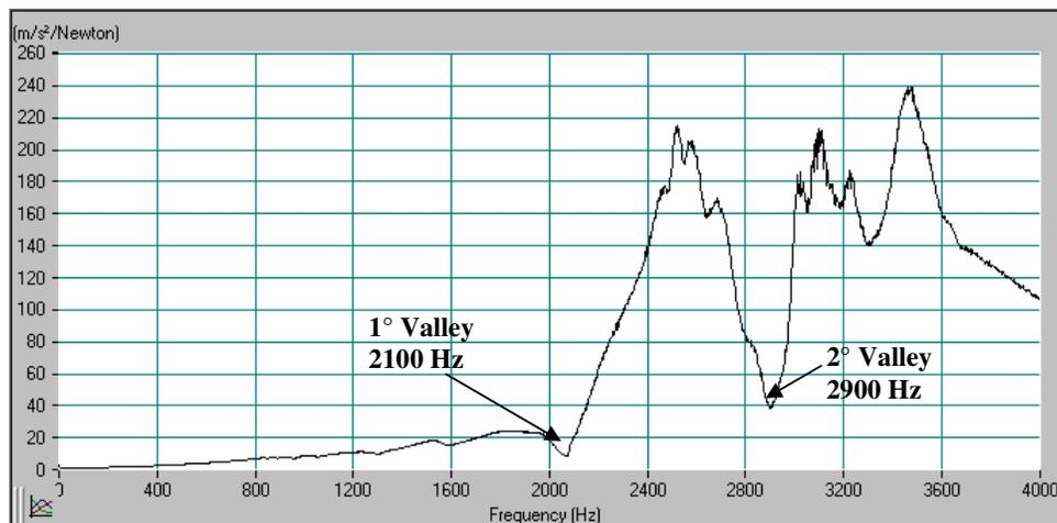
Figure 6. Selection of the first two valleys of the FRF of the assembly.
