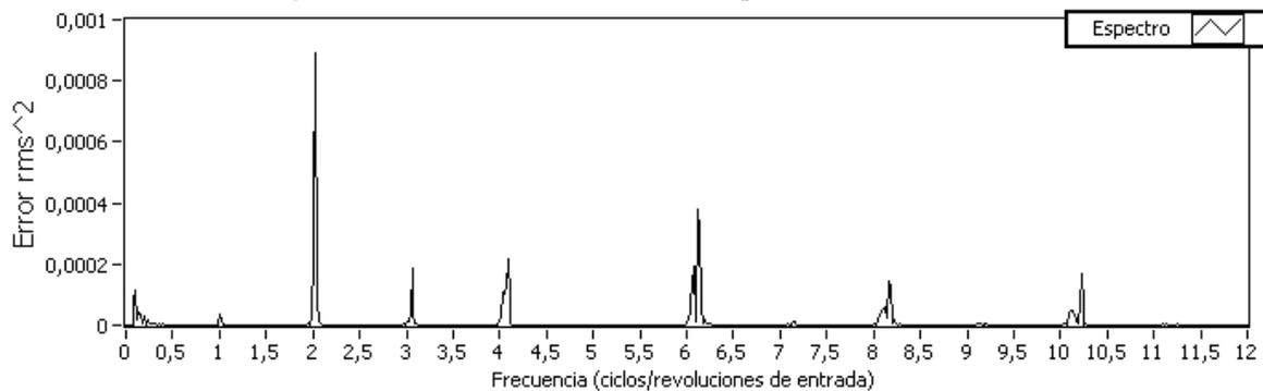
Figure 8. FFT of position error in cycles per input revolution at clockwise
