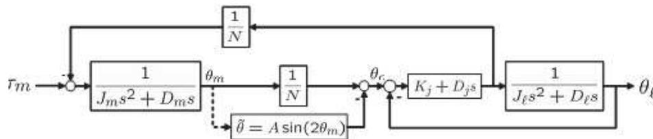
Figure 2. Non-linear model f HD into a motor model
