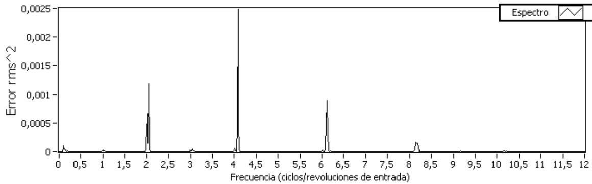
Figure 6. FFT of position error in cycles per input revolution (counterclockwise)
