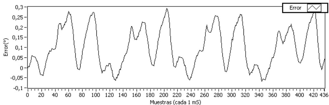
Figure 5. Position-error waveform at two input rotation (counterclockwise)
