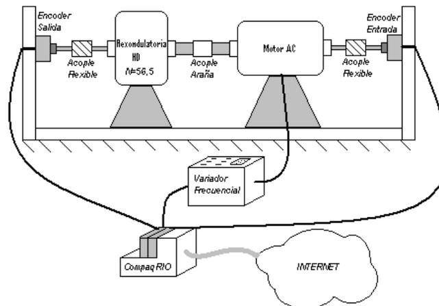
Figure 4. Scheme of Flexondulatoria (H. D.) testing apparatus
