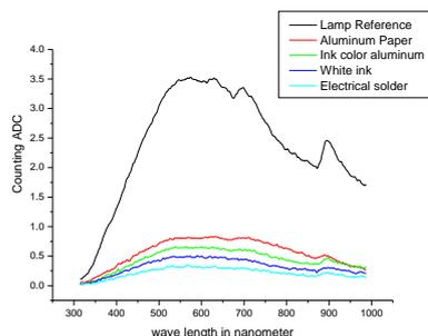
Figure 7. Reflecting pigments Photoacoustic absorption spectra
