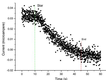
Figure 11. Temporal behavior of the prototype to have the lamp off
