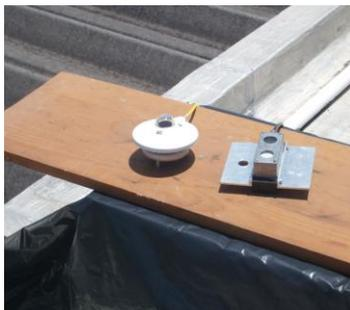
Figure 4. Kipp&Zonen and prototype under sunlight
