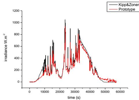
Figure 12. One day prototype and Kipp&Zonen sunlight measuring
