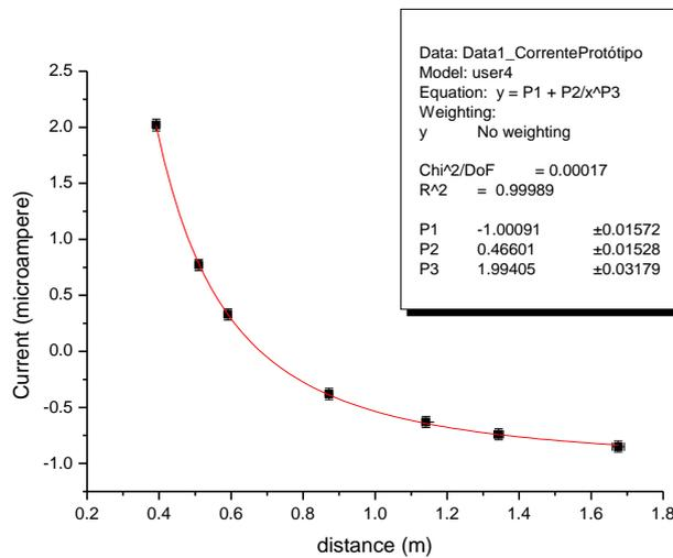
Figure 9. Variation of prototype electric signal as a function of the distance
