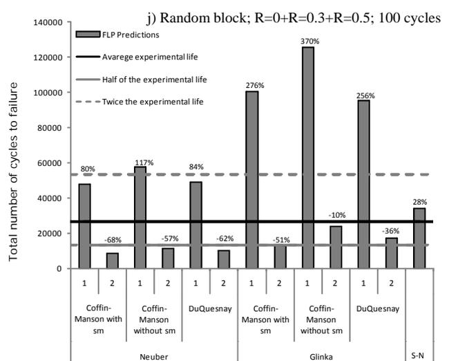
Figure 7. Fatigue life predictions for the variable amplitude block loading (continuation).
