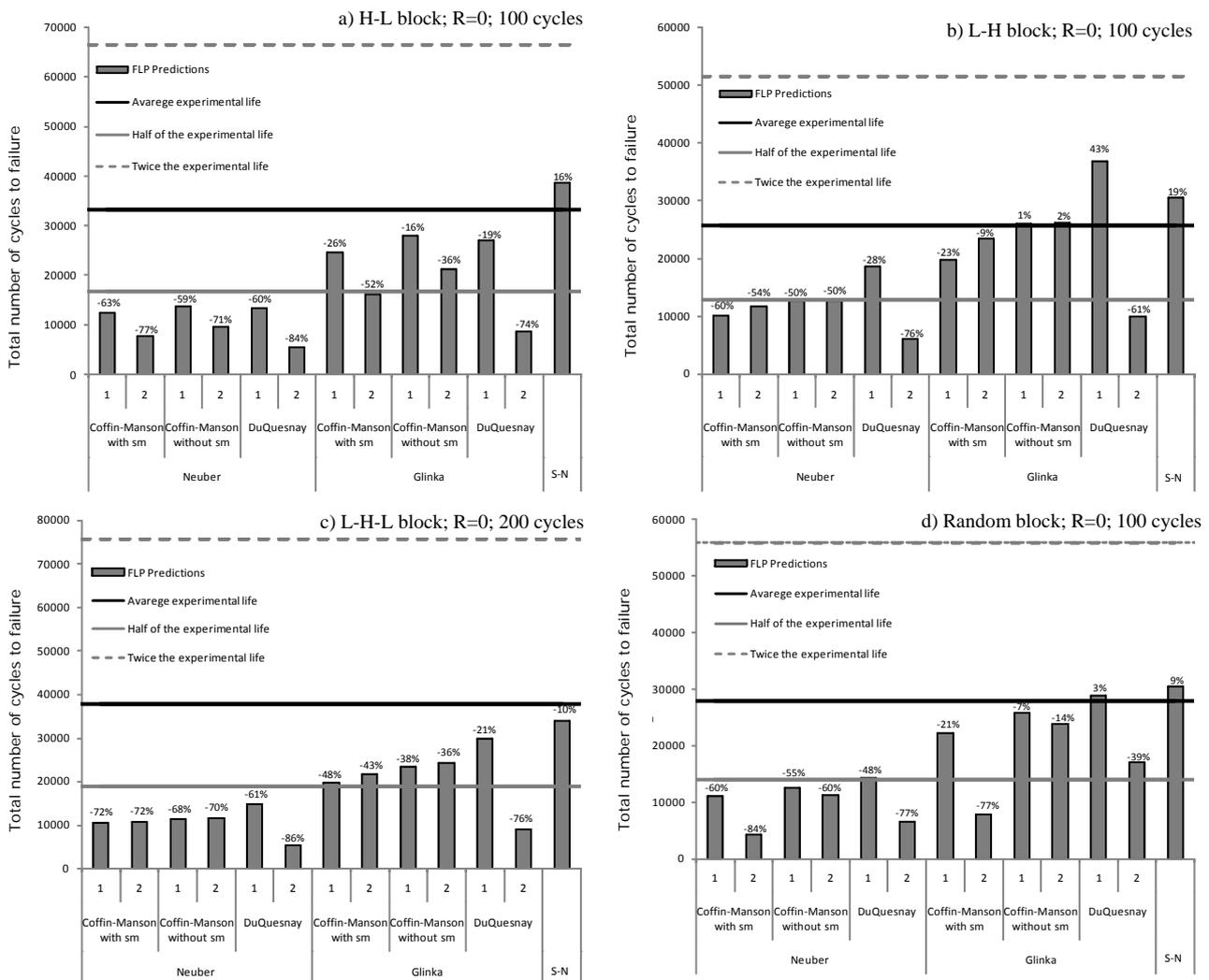
Figure 7. Fatigue life predictions for the variable amplitude block loading.
