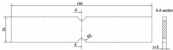
Figure 4. Geometry of the notched specimens (dimensions in mm).
