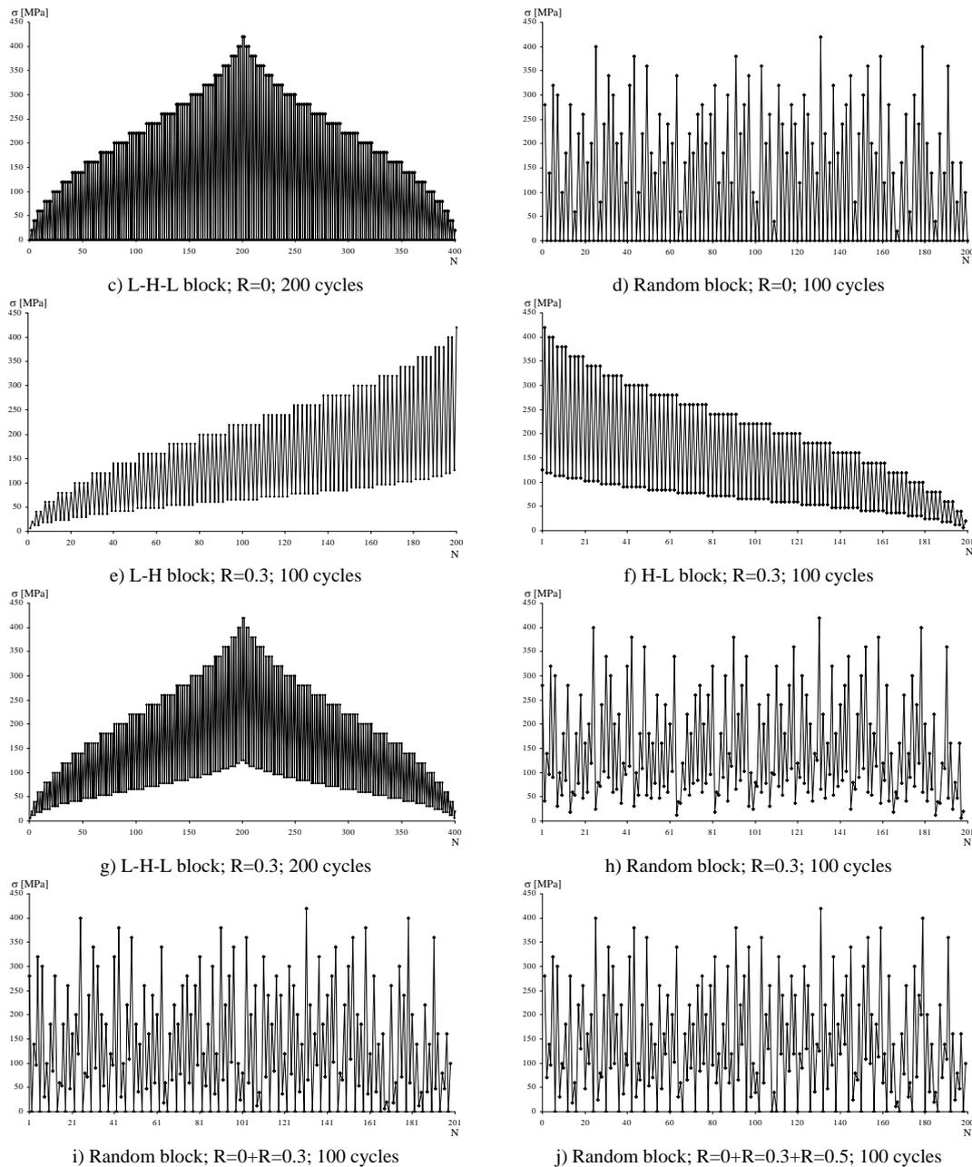
Figure 6. Variable amplitude blocks applied to the notched specimens (remote stress control) (continuation).
