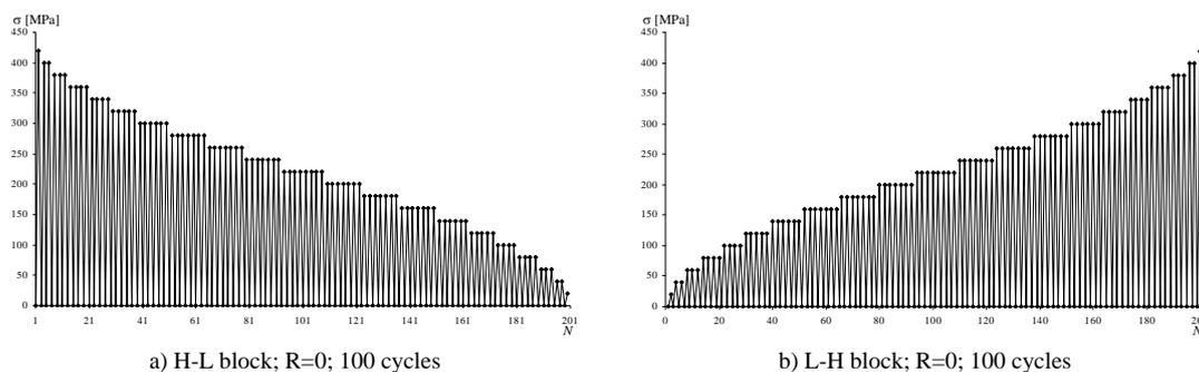
Figure 6. Variable amplitude blocks applied to the notched specimens (remote stress control).
