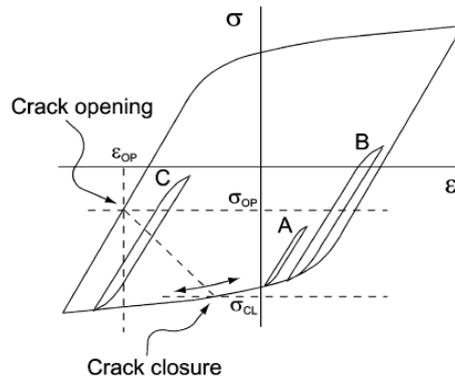
Figure 1. Crack opening *versus* crack closure behaviours (Lynn and DuQuesnay, 2002).
