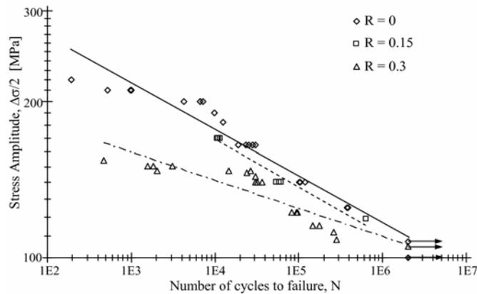
Figure 5. Constant amplitude S-N curves of the notched component ( $K_t=2.17$ ) made of P355NL1 steel (Pereira *et al.*, 2008b).
