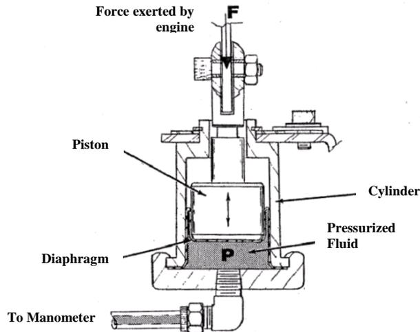
Figure 6. Original hydraulic load cell from Go-Power DY-7D Operating Manual.
