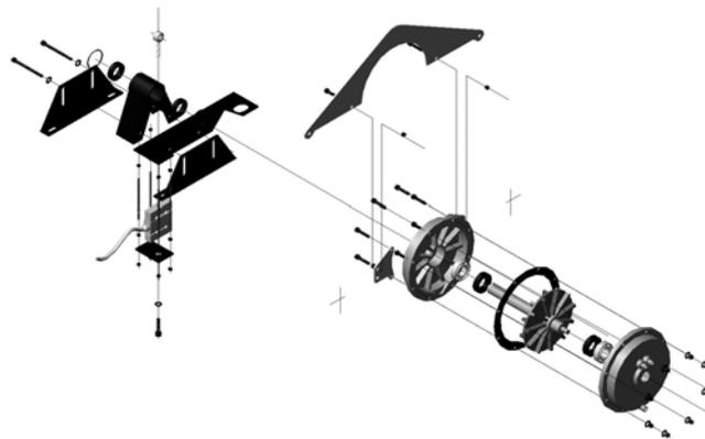
Figure 1 –Go-Power DY-7D Dynamometer - Exploded View
