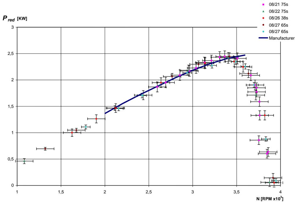
Figure10. Power vs RPM characteristic curve – Measured and manufacture data for Honda GX120T1
