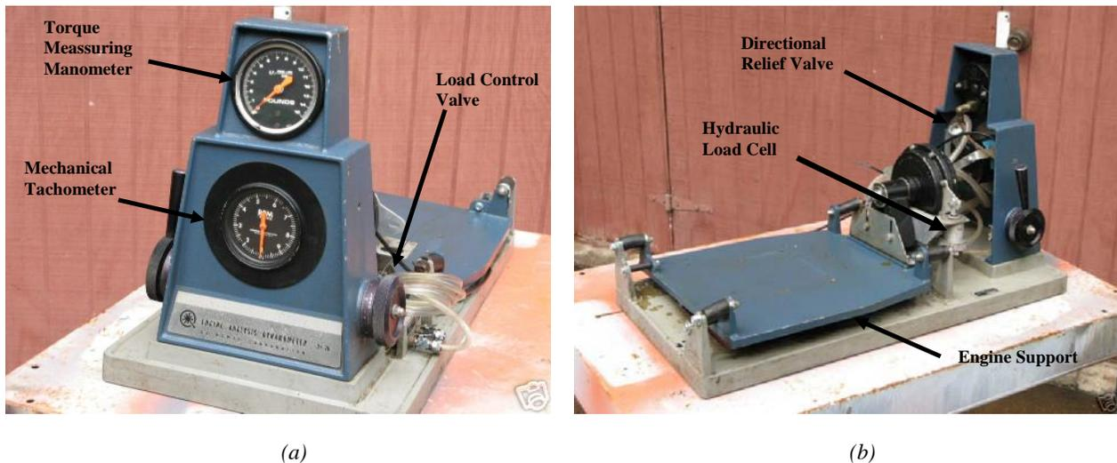
Figure 2 – Dynamometer Go-Power DY-7D – Frontal and Lateral views.
