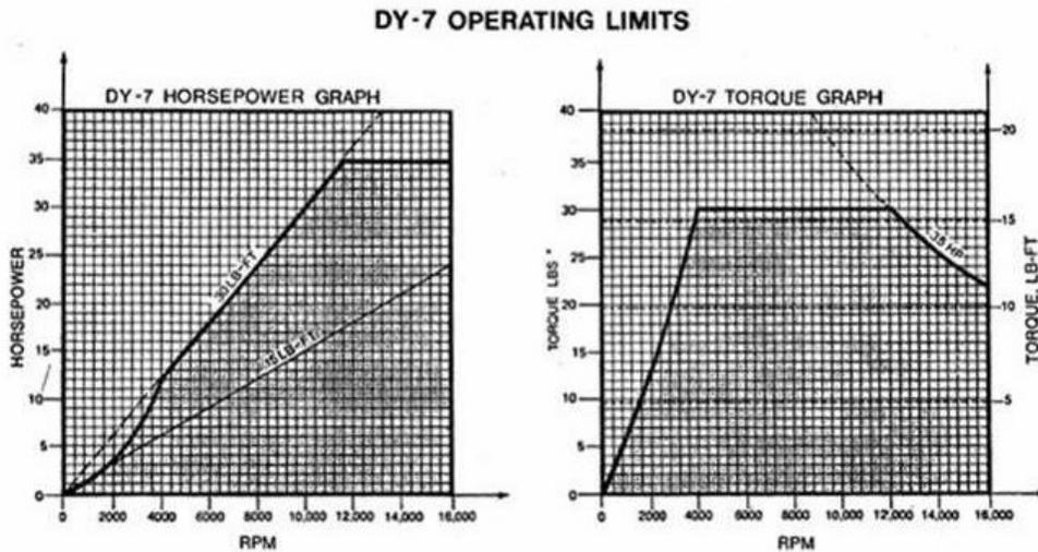
Figure 4 – Original dynamometer characteristic curves obtained from equipment manuals.
