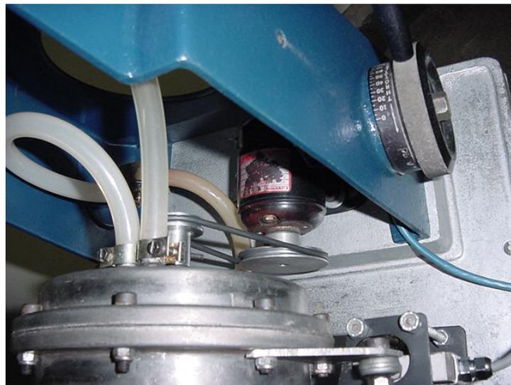
Figure 9. Final arrangement of the tachogenerator and the developed transmission system
