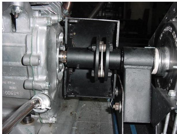
Figure 5. Disk coupling with flanges and protective case
