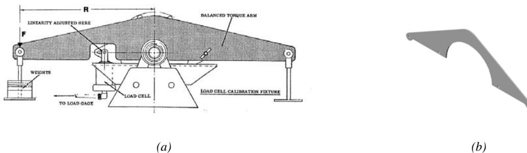
Figure 8. Sketch of the original calibration arm assembled in the dynamometer (a) GO-POWER DY-7D Operation Manual and of the proposed calibration arm (b).
