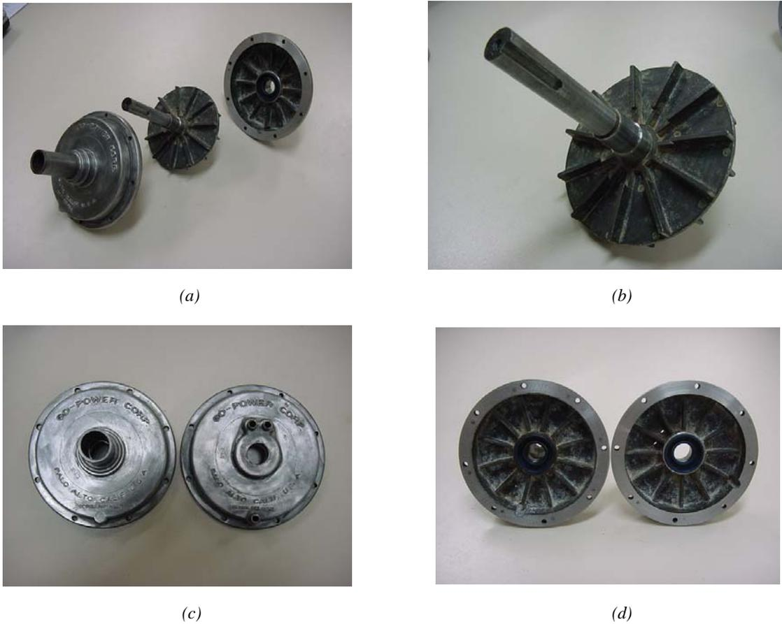
Figure 3 – Hydraulic Brake Interns - Rotor (a and b) and Casing (c and d) after maintenance
