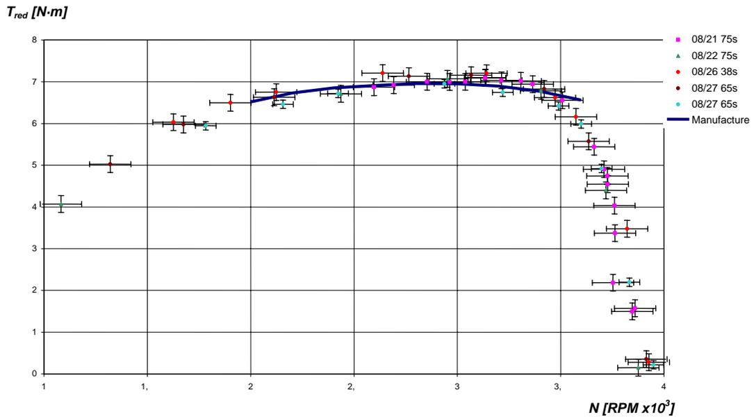
Figure10. Power vs RPM characteristic curve – Measured and manufacture data for Honda GX120T1
