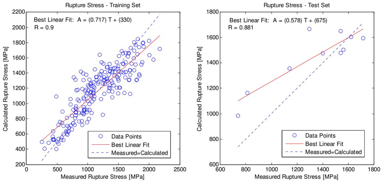
Figure 8: Predicted rupture stress by the neural network versus experimental values for (a) training and (b) test data sets.
