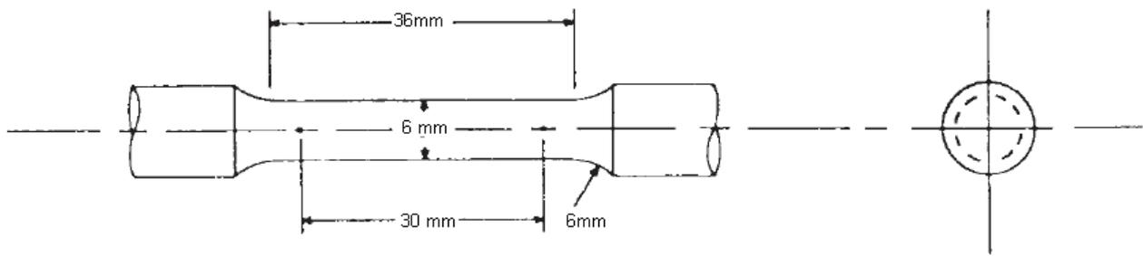
Figure 1: Specimen following the ASTM E8M standard for tensile testing.
