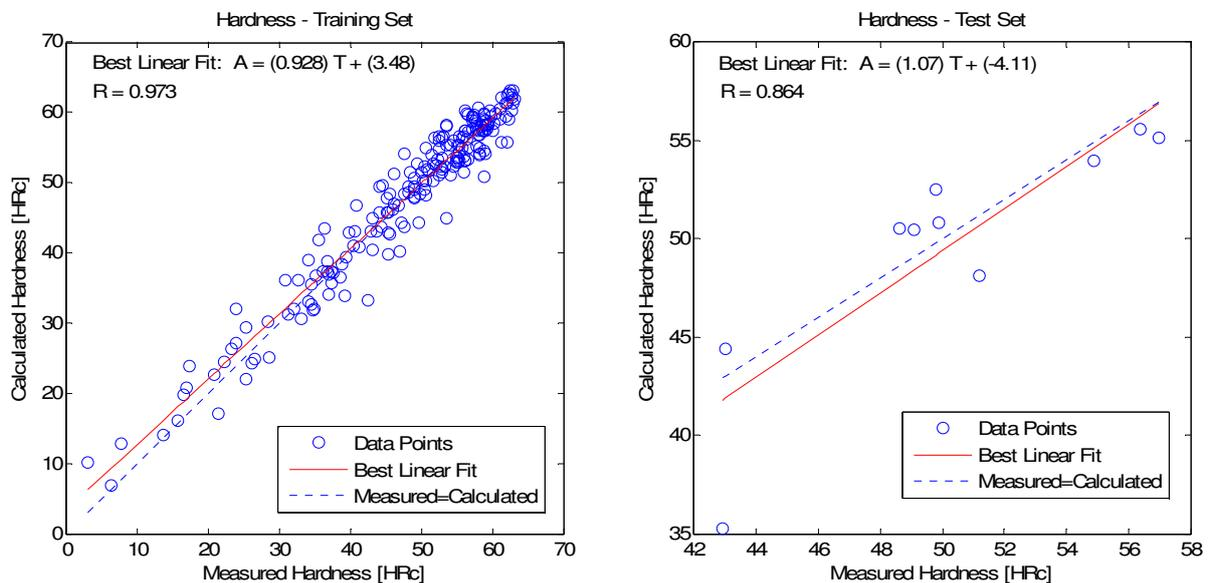
Figure 10: Predicted hardness by the neural network versus experimental values for (a) training and (b) test data sets.
