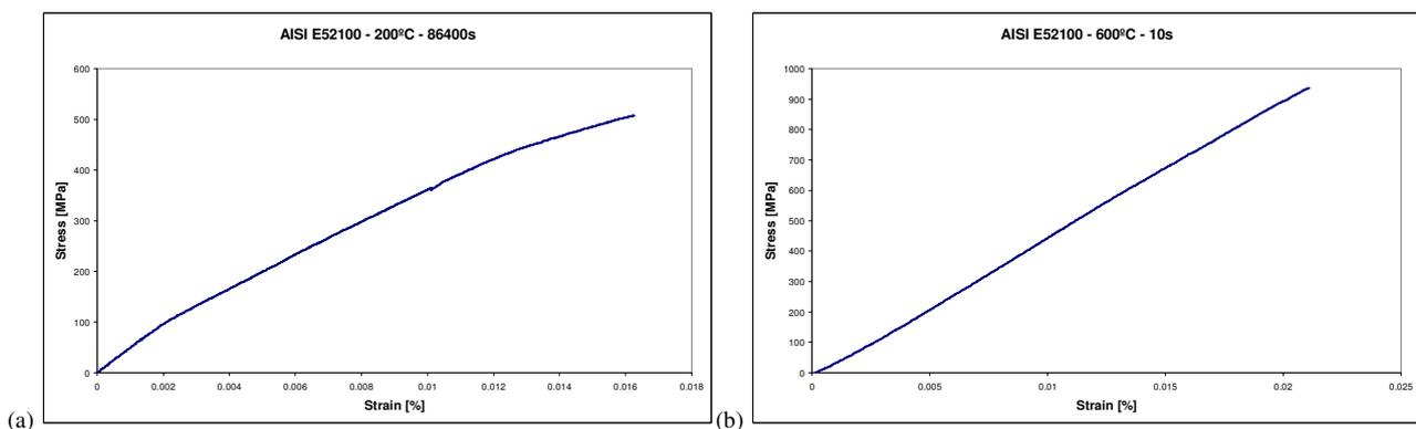
Figure 6: Stress-strain curve for AISI E52100 steel tempered for (a) 86400s at 200°C and (b) 10s at 600°C.
