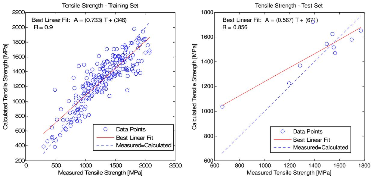
Figure 7: Predicted tensile strength by the neural network versus experimental values for (a) training and (b) test data sets.
