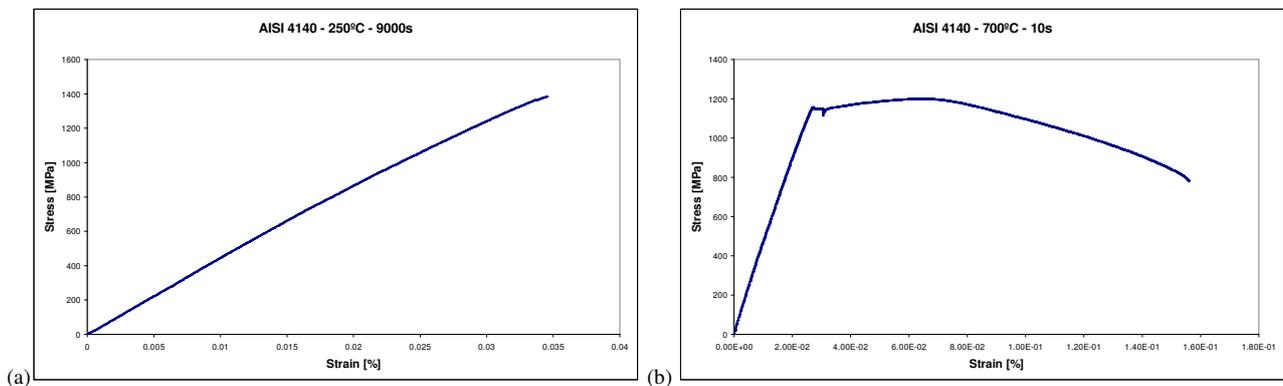
Figure 2: Stress-strain curve for AISI 4140 steel tempered for (a) 9000s at 250°C and (b) 10s at 700°C.
