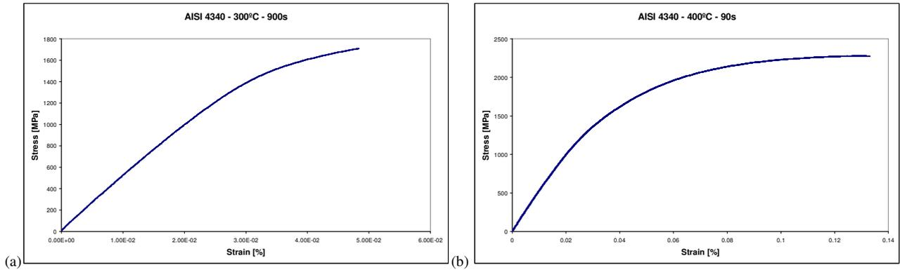
Figure 3: Stress-strain curve for AISI 4340 steel tempered for (a) 900s at 300°C and (b) 90s at 400°C.
