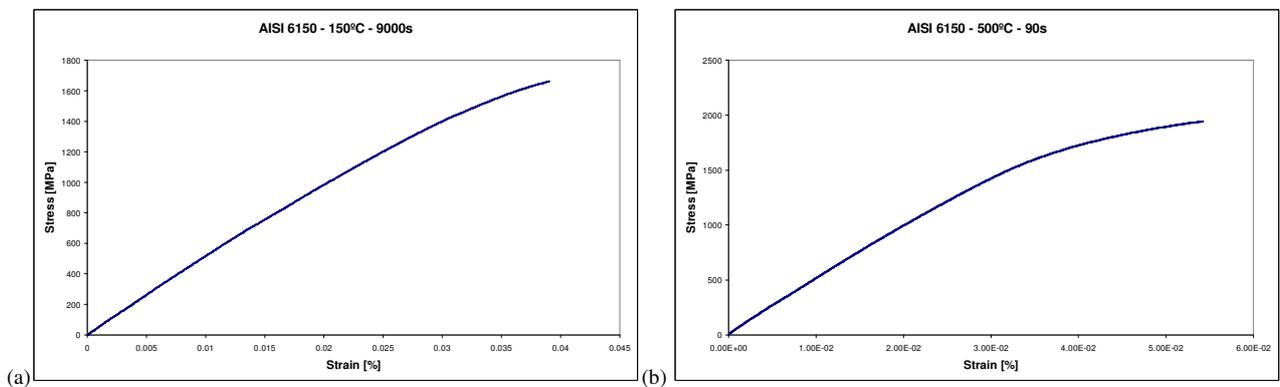
Figure 5: Stress-strain curve for AISI 6150 steel tempered for (a) 90000s at 150°C and (b) 90s at 500°C.
