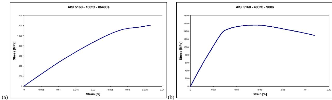
Figure 4: Stress-strain curve for AISI 5160 steel tempered for (a) 86400s at 100°C and (b) 300s at 400°C.
