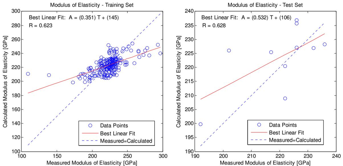
Figure 9: Predicted modulus of elasticity by the neural network versus experimental values for (a) training and (b) test data sets.
