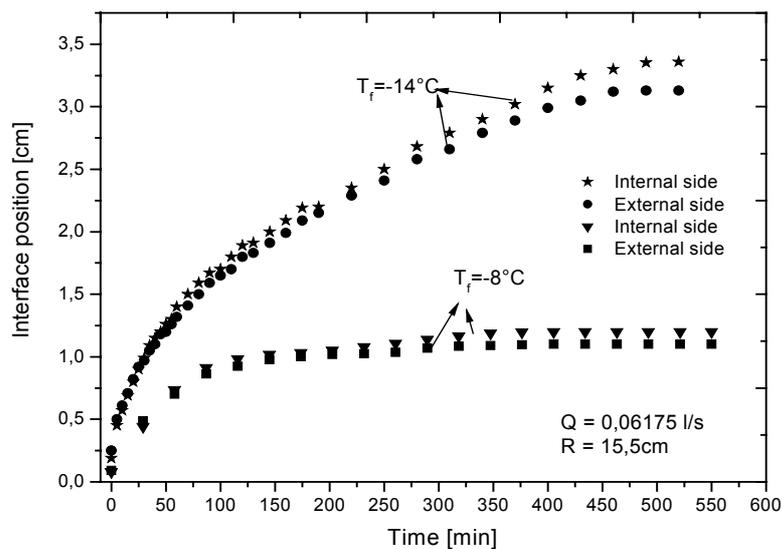
Figure 4 Variation of the interface position with time.
