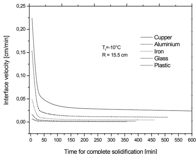
Figure 12 Effect of the curved tube material on the time for complete solidification.
