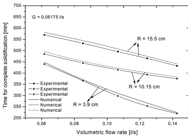
Figure 10 Effects of the volumetric flow rate on the time for complete solidification.
