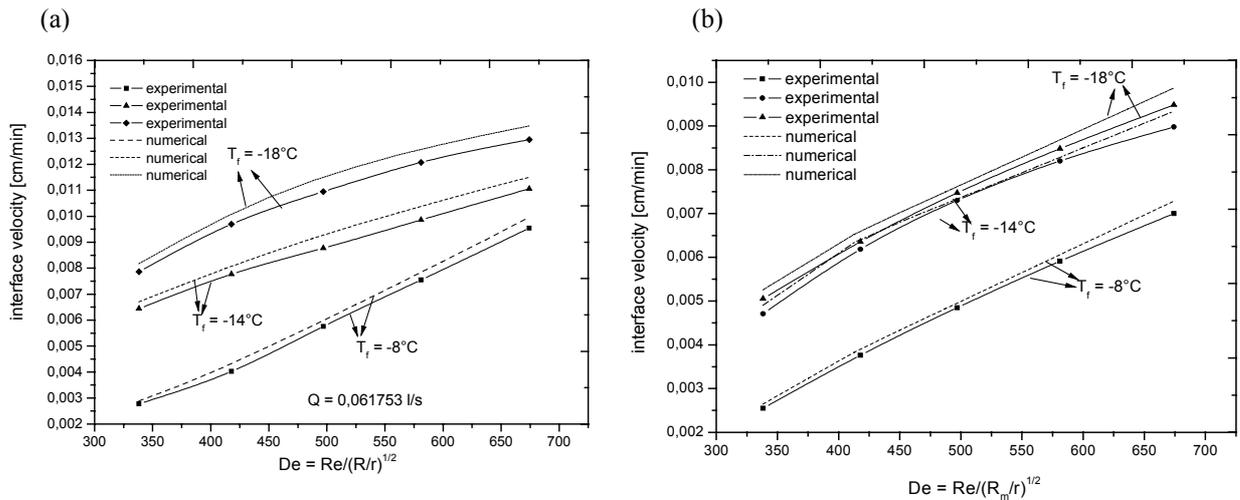
Figure 7 (a) Effects of the Dean number on the interface velocity on the internal side of the curved tube. (b) Effects of the Dean number on the interface velocity on the external side of the curved tube
