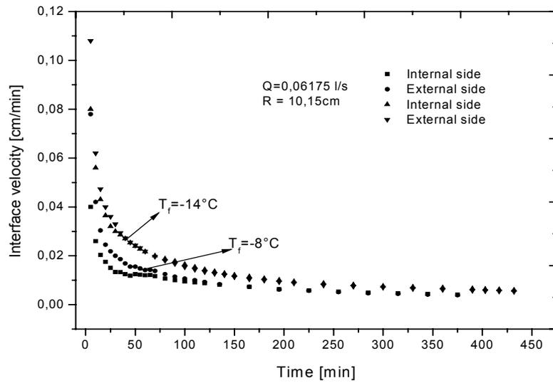
Figure 5 Variation of the interface velocity as a function of time.
