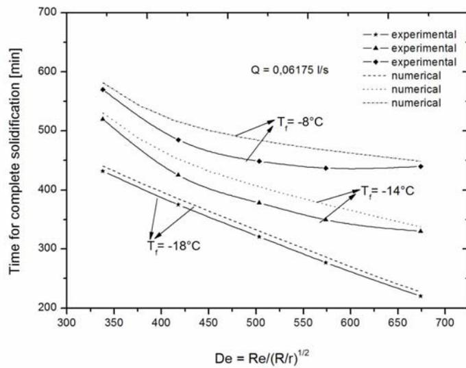
Figure 9 Effects of the Dean number on the time for complete solidification.
