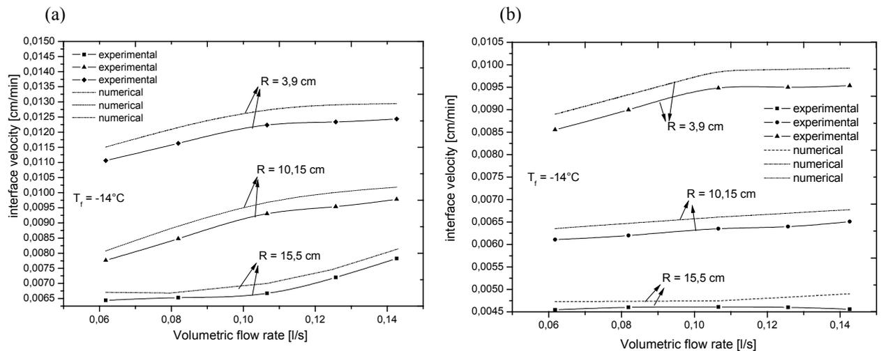
Figure 8 (a) Effects of the volumetric flow rate on the interface velocity on the internal side of the curved tube. (b) Effects of the volumetric flow rate on the interface velocity on the external side of the curved tube.
