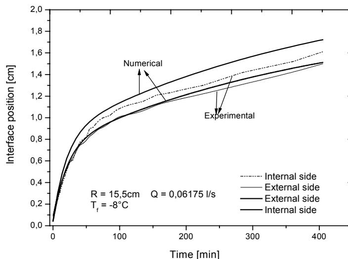
Figure 6 Comparison between the numerical predictions and experimental results.
