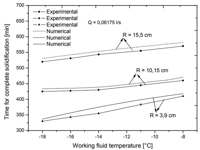
Figure 11 Effects of the working fluid temperature on the time for complete solidification
