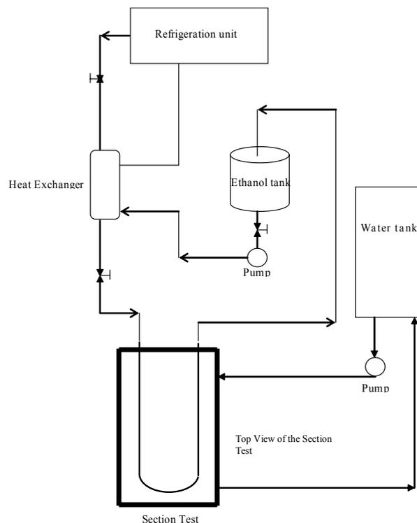
Figure 1 – Scheme diagram of the experimental setup
