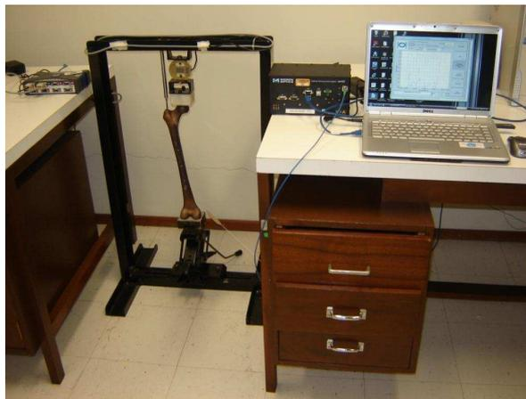
Figure 3: Test arrangement and instrumentation of the femur
