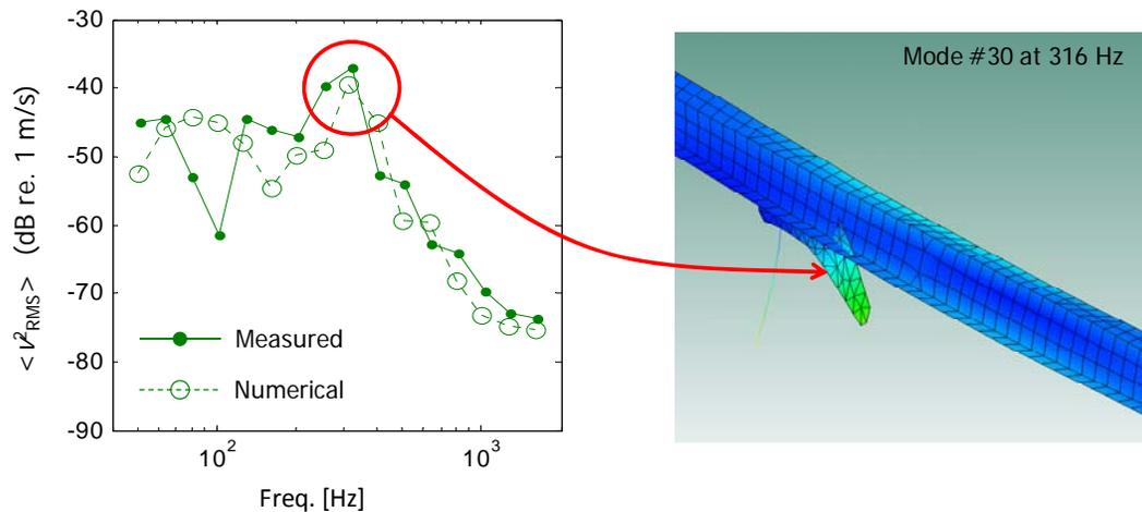
Figure 8. RMS velocity of the top panel of the bin due to point force excitation at the end of the tie rod (Cotoni *et al*, 2008).
