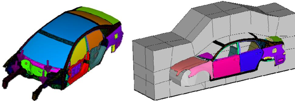
Figure 1. Hybrid FE-SEA model of a vehicle for structure-borne excitations (Charpentier *et al* 2008a).
