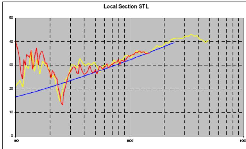
Figure 6. Transmission loss of a region of the dash panel – Numerical results (red), experimental results (yellow) and mass-law curve (blue) (Shorter *et al.*, 2007).
