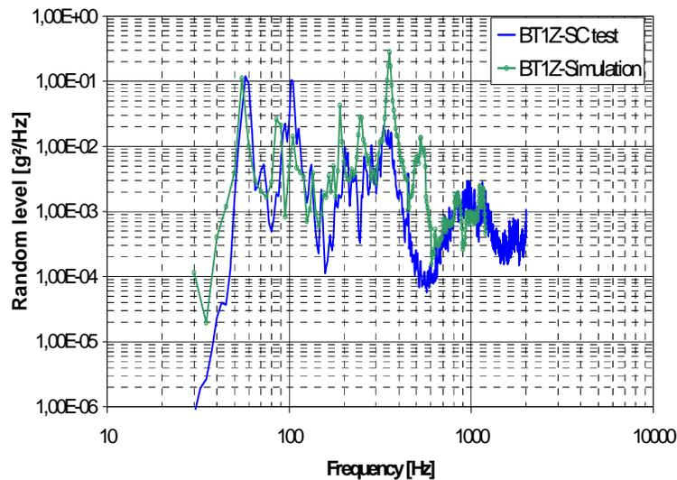
Figure 4. Vibrational response of a component of the satellite due to a diffuse acoustic field environment— Experimental vs. simulated results (Knockaert *et al*, 2007).
