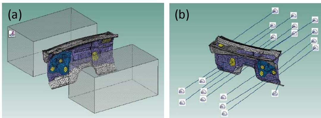
Figure 5: Hybrid FE-SEA of a vehicle dash panel. (a) Chambers as SEA cavities; (b) – Chambers as energy sinks (SEA semi-infinite fluids) (Shorter *et al*, 2007).
