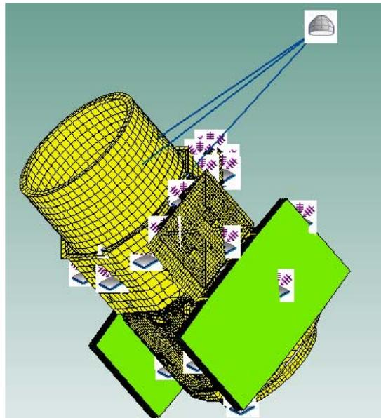
Figure 3. Hybrid FE-SEA model of a satellite (Knockaert *et al*, 2007).
