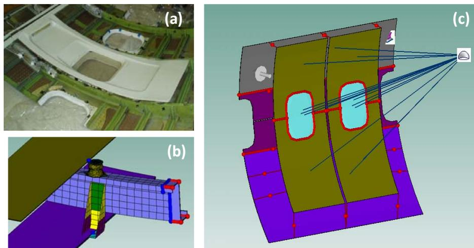
Figure 9. (a) Fuselage and interior panel considered in the analysis; (b) Hybrid FE-SEA component level model; and (c) SEA system level models.
