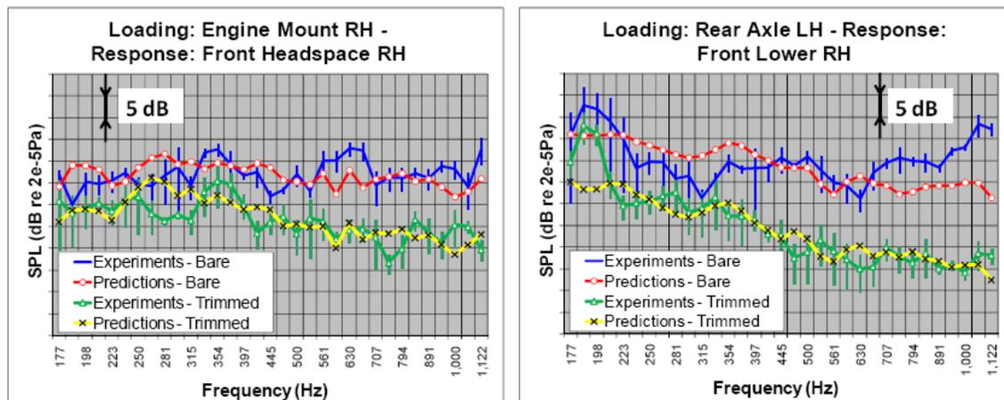
Figure 2. Sound pressure inside the vehicle for excitation at the engine mount (left) and at the rear axle (right) without the sound package (bare) and after its installations (trimmed) - Hybrid vs. experimental (Charpentier *et al* 2008b).
