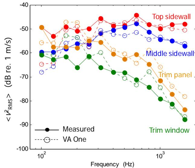
Figure 10. RMS velocity of subsystems of the SEA system level model.
