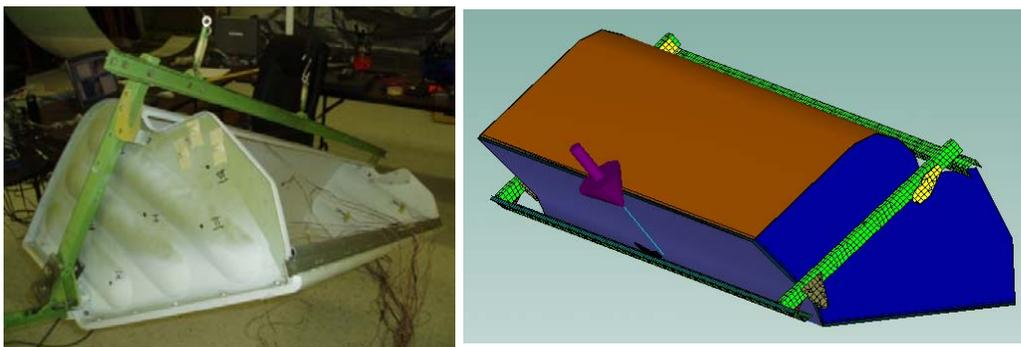
Figure 7. Overhead bin and corresponding Hybrid FE-SEA model (Cotoni *et al.*, 2008).
