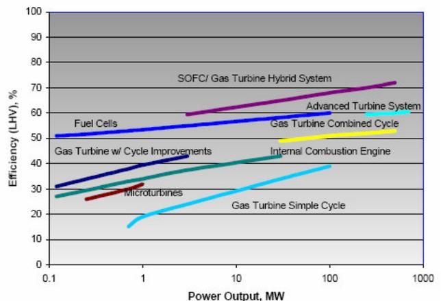
Figure 8. Estimated Efficiency of Different Power Generation Systems, by Eg&G Technical Services (2004)
