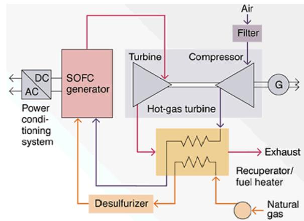
(b) System diagram for the 300kW class SOFC-GT hybrid cycle system.
