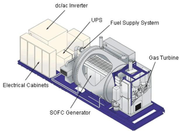
(a) The SOFC is shown in the middle of the diagram, and operates at about 10 bar inside the cylindrical pressure vessel. The gas turbine, compressor, and alternator are behind the fuel cell.
