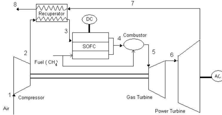
Figure 3. Schematic of a combined Gas Turbine power plant with an SOFC (Haseli *et al.* (2008)).
