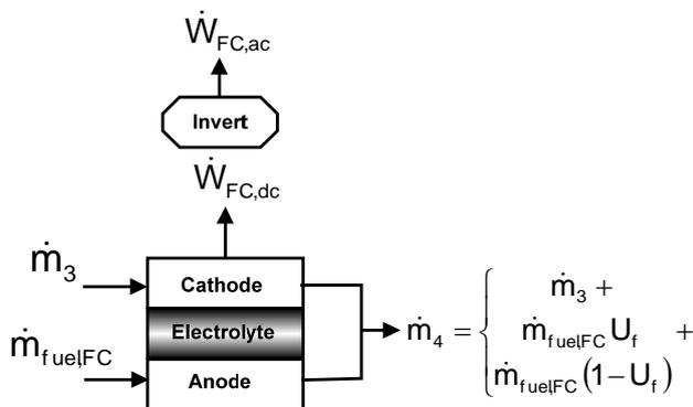
Figure 4. Schematic of the SOFC cell showing the inlet and outlet flows, Haseli *et al.* (2008).
