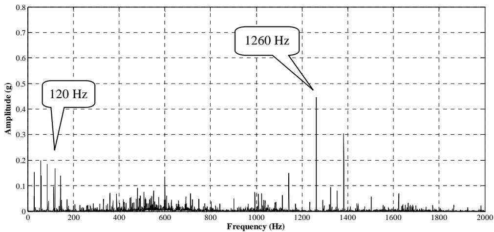
Figure 10. Vibration spectrum with ten turns short circuited.
