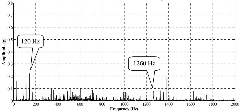
Figure 6. Vibration spectrum without fault with the machine operating at rated speed and rated load.
