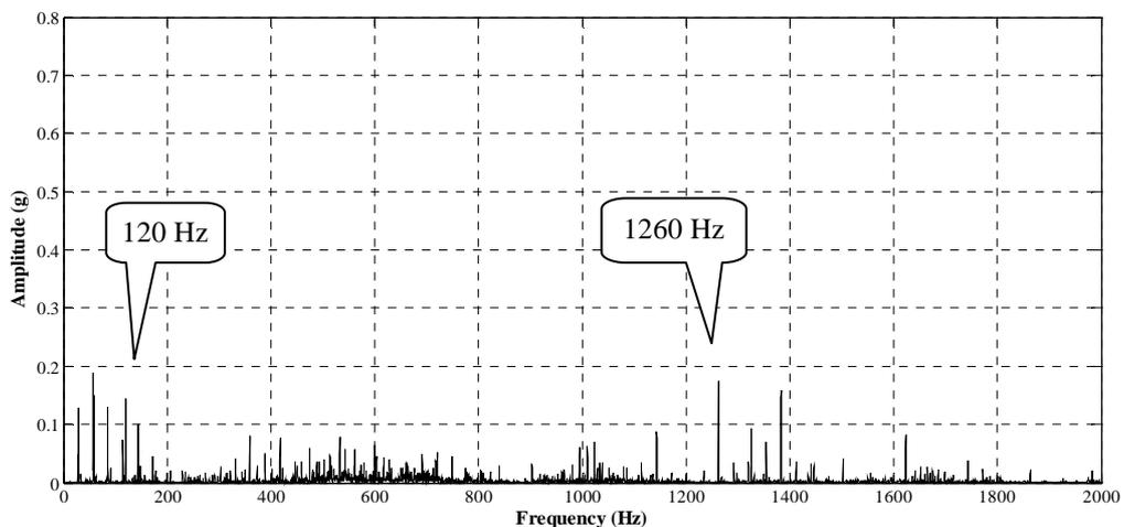
Figure 8. Vibration spectrum with four turns short circuited.
