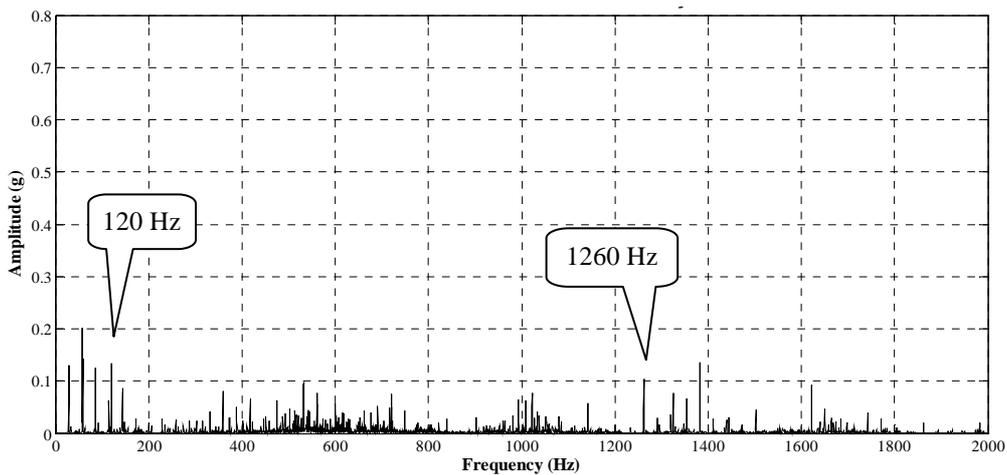
Figure 7. Vibration spectrum with two turns short circuited.
