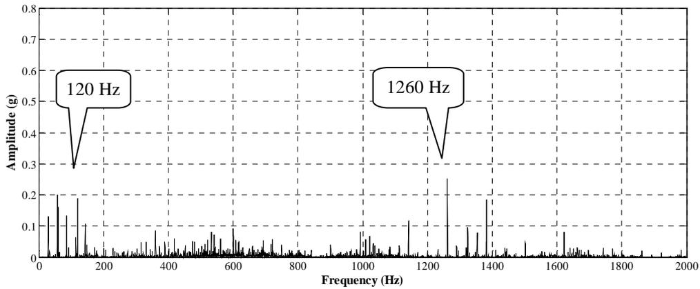
Figure 9. Vibration spectrum with six turns short circuited.
