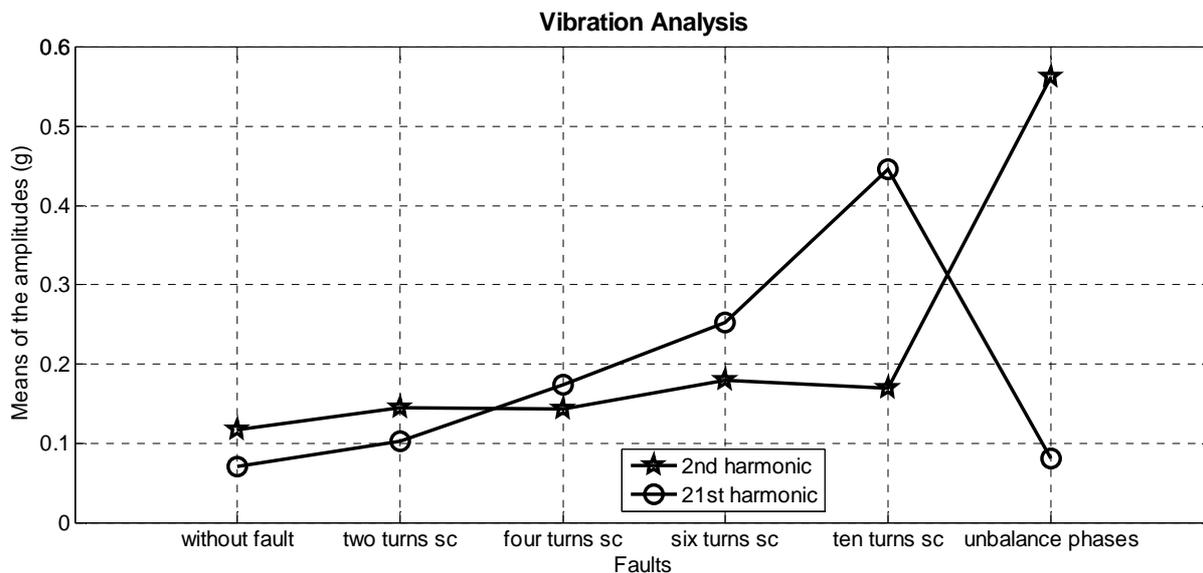
Figure 12. Tendency of introduces faults.
