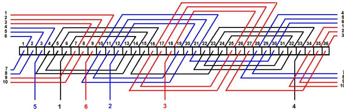
Figure 3 - Stator winding arrangement.
