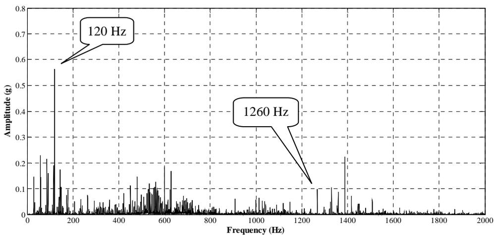
Figure 11. Vibration spectrum with unbalance phase.
