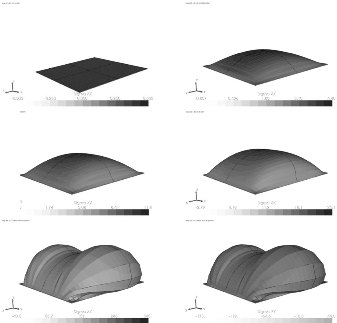
Figure 3. Sequence of configurations in the membrane.
