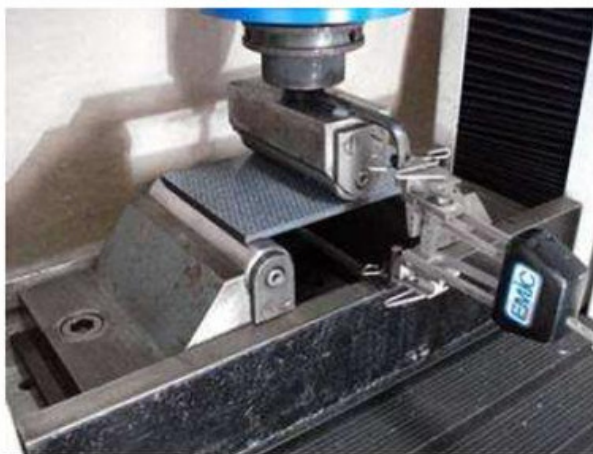
Figure 4. 3PF device utilized to determine the residual monotonic properties of the impacted laminates.
