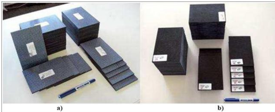
Figure 1. Sets of CAI test specimens: (a) Thermoplastic PPS-C laminate; (b) Thermosetting EPX-C composite.
