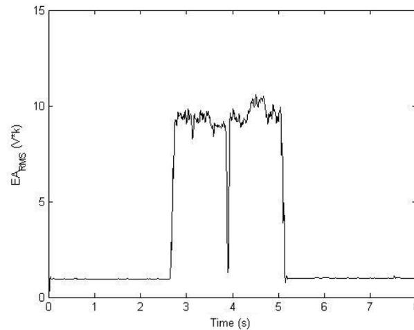
Figure 7. Pass 1 from test 7,  $a_d = 40 \mu\text{m}$ , with cutting fluid
