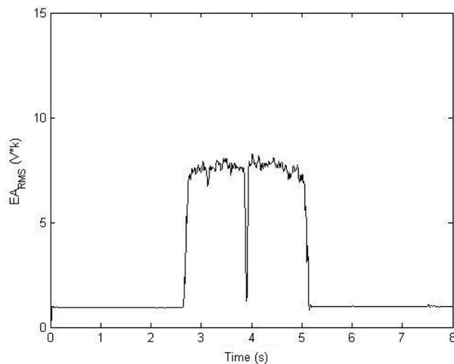
Figure 10. Pass 1 from test 7,  $a_d = 40 \mu\text{m}$ , with cutting fluid, filtered with a cutoff frequency of 70 kHz
