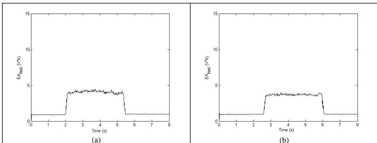
Figure 9. Pass 1 (a) and 14 (b) from test 3,  $a_d = 20 \mu\text{m}$ , with cutting fluid, filtered with a cutoff frequency of 70 kHz
