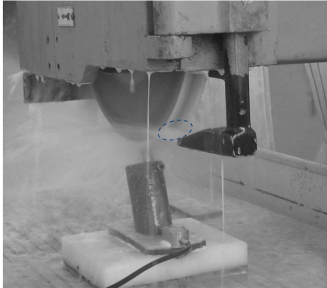
Figure 2. Irregular cutting fluid flow during dressing operation
