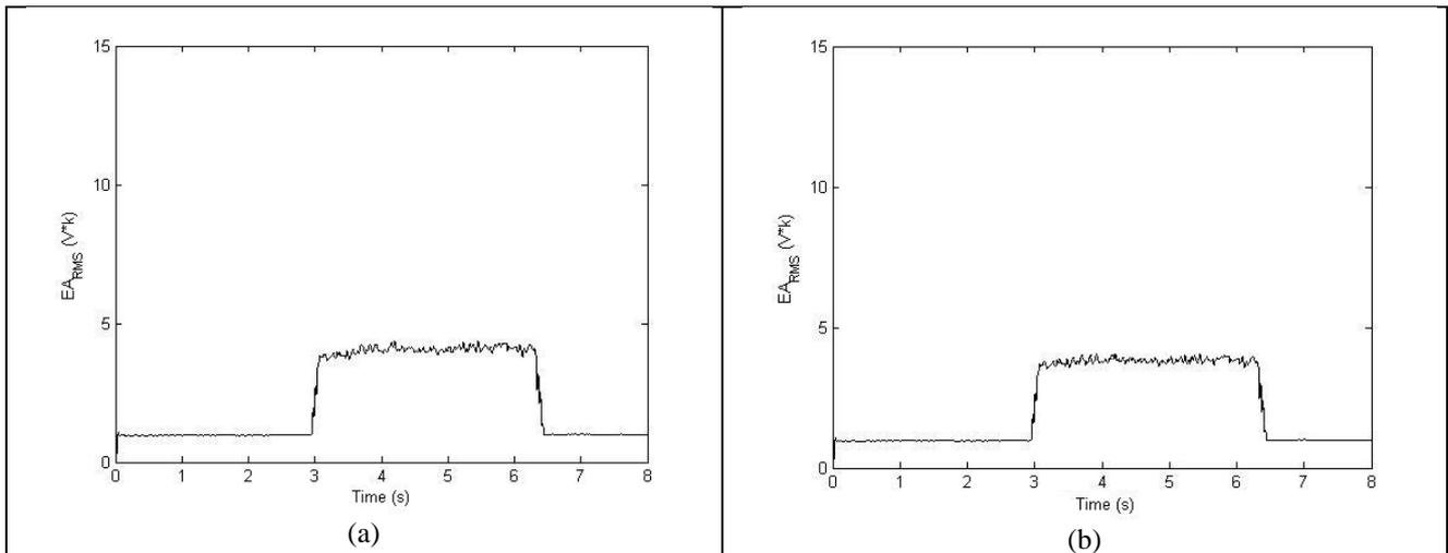
Figure 8. Pass 5 from test 3,  $a_d = 20 \mu\text{m}$ , filtered with a cutoff frequency of 60 kHz (a) and 70 kHz (b)
