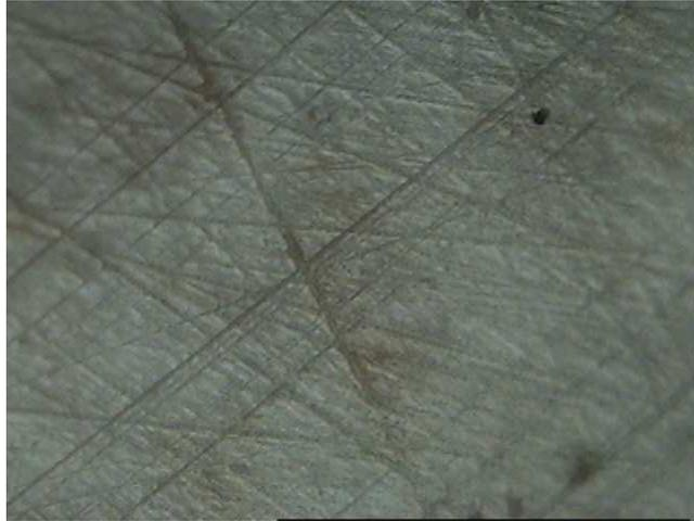
Figure 4. Ceramic submerged in ocean petroleum for 15 days
