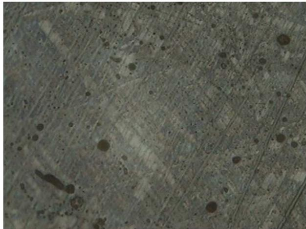
Figure 5. Ceramic submerged in ocean petroleum for 30 days
