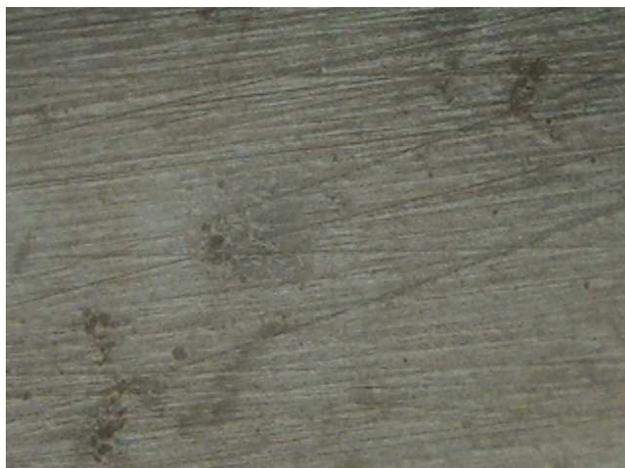
Figure 6. Ceramic submerged in ocean petroleum for 15 days
