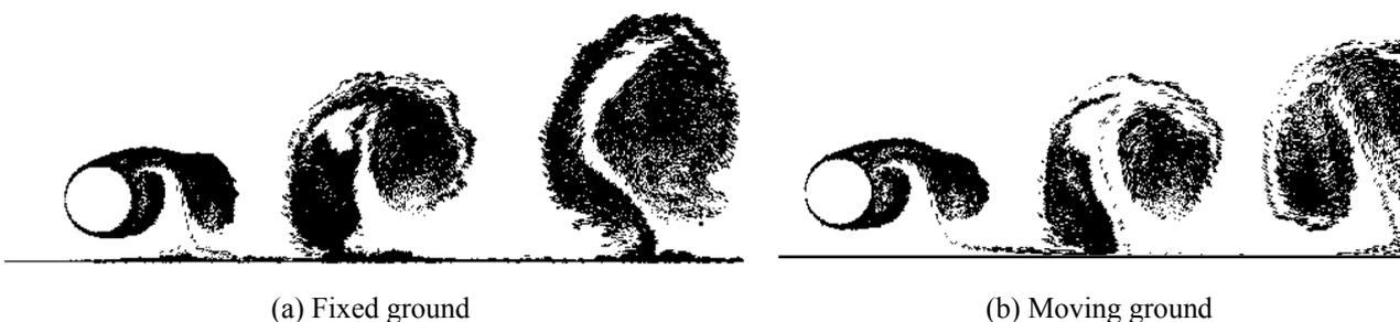
Figure 7. Near field velocity distribution at an instant represented by point C;  $Re=1.0 \times 10^5$  and  $h/d=0.45$
