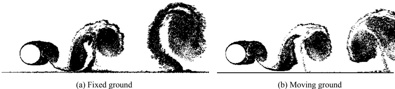
Figure 6. Near field velocity distribution at an instant represented by point B;  $Re=1.0 \times 10^5$  and  $h/d=0.45$
