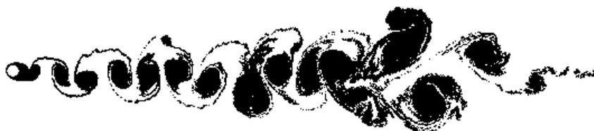
Figure 9. Position of the wake vortices at  $t=50$  for an isolated cylinder case;  $Re=1.0 \times 10^5$  and  $h/d \rightarrow \infty$ .
