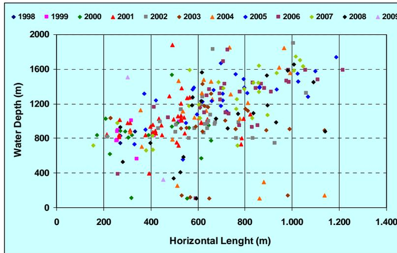
Figure 1. Typical Horizontal lengths of Brazilian wells
