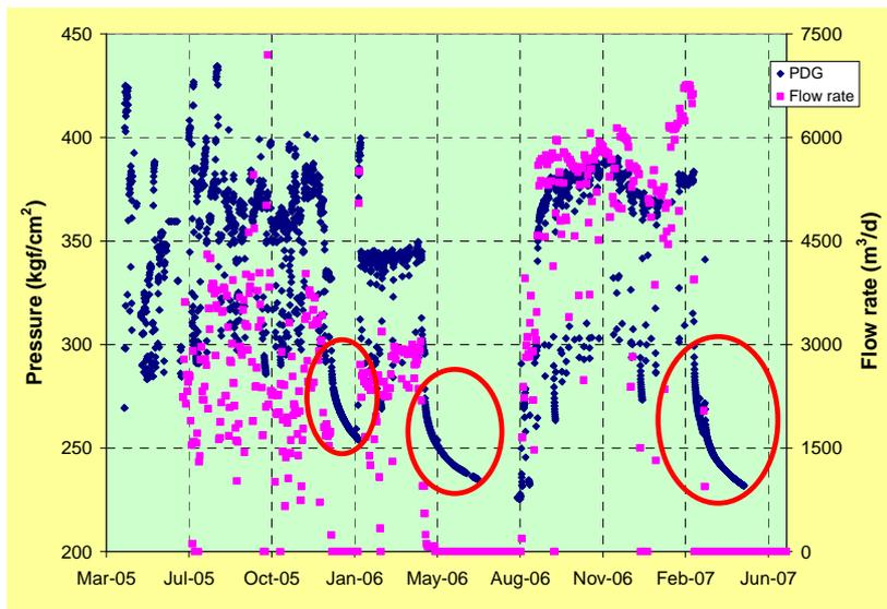
Figure 4. Identifying fall of periods of an injection well
