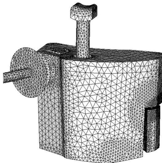
Figure 3. Computational grid for the three-dimensional formulation.
