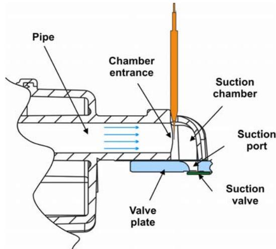
Figure 2. Detail of anemometry sensor assembly.
