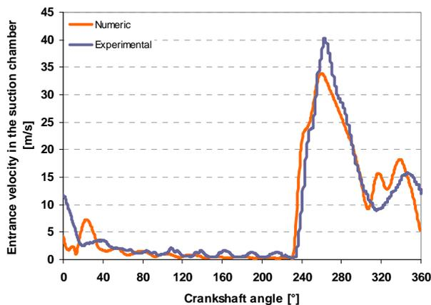
Figure 4. Instantaneous velocity in the suction chamber.
