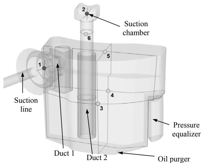
Figure 1. Suction muffler geometry and measurement positions.
