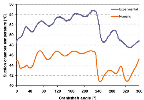
Figure 5. Instantaneous temperature in the suction chamber.
