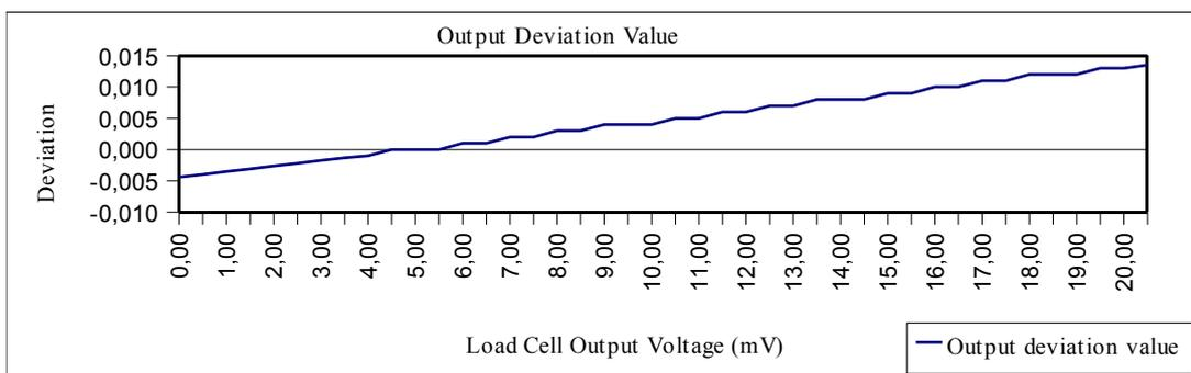
Figure 8. Output Deviation Value for Signal Conditioning
