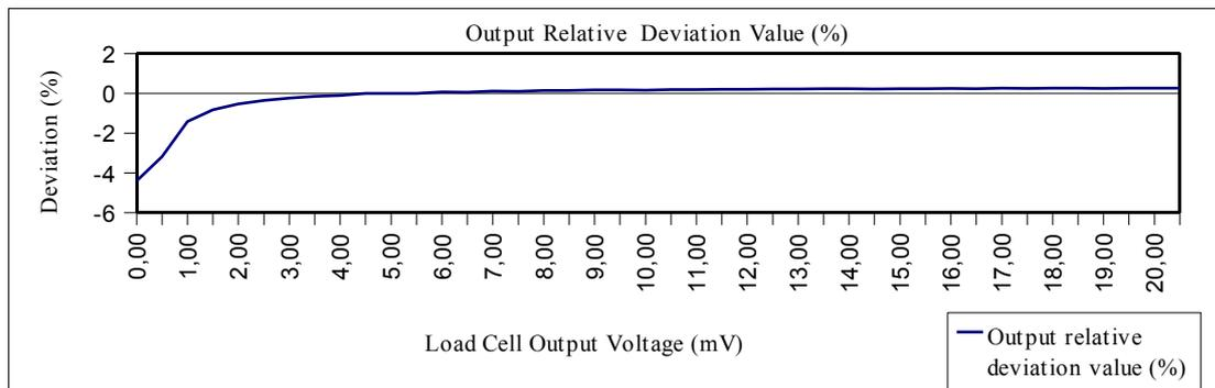
Figure 9. Output Relative Deviation Value in percentage for Signal Conditioning
