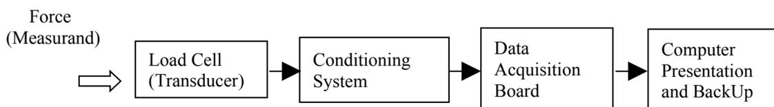
Figure 3. Measuring System Block Diagram
