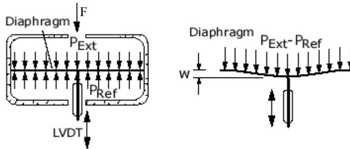
Figure 5. Diagram of LVDT Load Cell Operation
