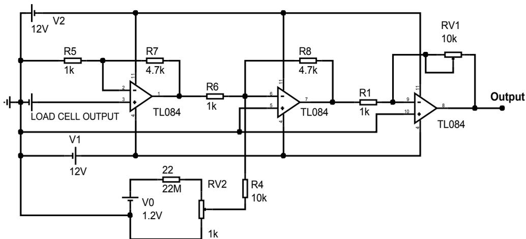
Figure 6. Signal Conditioning Electronic Circuit
